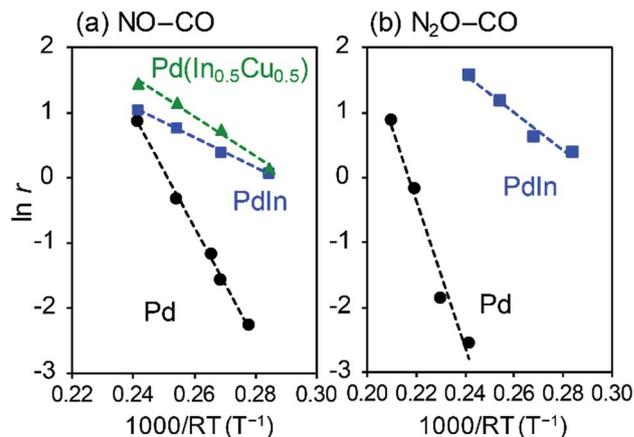
Fig. 8 Arrhenius-type plots for (a) NO and (b)  $N_2O$  reduction by CO using Pd/Al<sub>2</sub>O<sub>3</sub>, PdIn/Al<sub>2</sub>O<sub>3</sub>, and Pd(In<sub>0.5</sub>Cu<sub>0.5</sub>)/Al<sub>2</sub>O<sub>3</sub> catalysts. Reaction rates (mol s<sup>-1</sup> mol<sub>Pd</sub><sup>-1</sup>) are evaluated based on the CO<sub>2</sub> formation rate.
