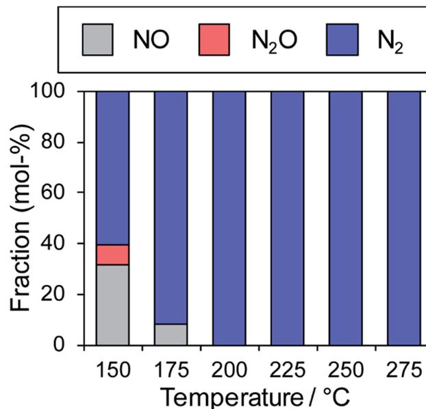
Fig. 6 Fraction of NO, N<sub>2</sub>O and N<sub>2</sub> in effluent gas (mol%) during catalytic NO reduction with CO using the Pd(In<sub>0.33</sub>Cu<sub>0.67</sub>)/Al<sub>2</sub>O<sub>3</sub> catalyst (NO and CO: 0.5% balanced with He; catalyst: 0.060 g; total flow: 48 ml min<sup>-1</sup>).
