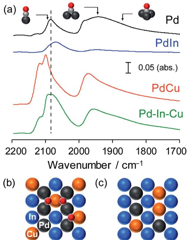
Fig. 4 (a) FT-IR spectra of CO adsorbed on Pd/Al<sub>2</sub>O<sub>3</sub>, PdIn/Al<sub>2</sub>O<sub>3</sub>, PdCu/Al<sub>2</sub>O<sub>3</sub> and Pd-In-Cu/Al<sub>2</sub>O<sub>3</sub> (Pd : In : Cu = 3 : 1 : 2) catalysts. Atomic arrangement of the most stable (110) surface of Pd(In<sub>1-x</sub>Cu<sub>x</sub>) assuming (b) In-Cu and (c) Pd-Cu replacement. Pd<sub>2</sub>Cu hollow sites are formed in (b).
