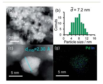
Fig. 1 (a) HAADF-STEM image of PdIn/Al $_2$ O $_3$  and (b) size distribution of the nanoparticles. (c) High-resolution STEM image of a single nanoparticle and (d) elemental maps of Pd and In in the nanoparticle acquired using EDX.
