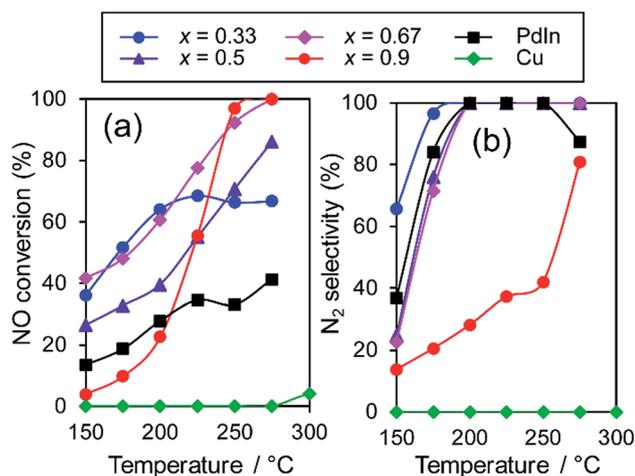
Fig. 5 Temperature dependence of NO conversion and N<sub>2</sub> selectivity in NO reduction by CO over various Pd–In–Cu/Al<sub>2</sub>O<sub>3</sub> (Pd : In : Cu = 1 : 1– $x$  :  $x$ ) catalysts.
