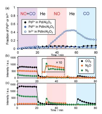
Fig. 9 (a) Changes in the fraction of Pd<sup>2+</sup> and In<sup>3+</sup> species in Pd and PdIn catalysts during contact with NO + CO, NO, and CO at 200 °C. The corresponding changes in the product distribution in the gas phase for (b) Pd and (c) PdIn are also shown.
