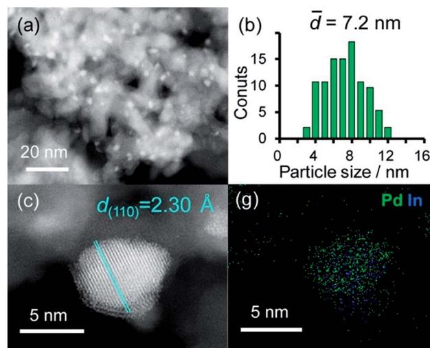
Fig. 1 (a) HAADF-STEM image of PdIn/Al<sub>2</sub>O<sub>3</sub> and (b) size distribution of the nanoparticles. (c) High-resolution STEM image of a single nanoparticle and (d) elemental maps of Pd and In in the nanoparticle acquired using EDX.
