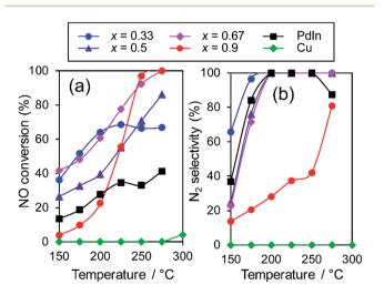
Fig. 5 Temperature dependence of NO conversion and N $_2$  selectivity in NO reduction by CO over various Pd-In-Cu/Al $_2$ O $_3$  (Pd : In : Cu = 1 : 1-x : x) catalysts.
