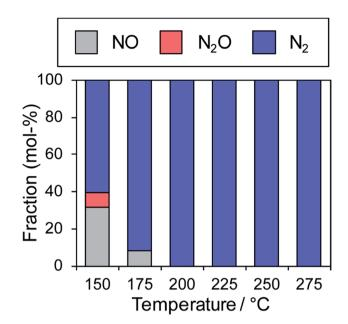
Fig. 6 Fraction of NO, N<sub>2</sub>O and N<sub>2</sub> in effluent gas (mol%) during catalytic NO reduction with CO using the  $Pd(In_{0.33}Cu_{0.67})/Al_2O_3$  catalyst (NO and CO: 0.5% balanced with He; catalyst: 0.060 g; total flow: 48 ml min<sup>-1</sup>).
