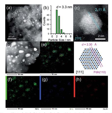
Fig. 3 (a) HAADF-STEM image of  $Pd-In-Cu/Al_2O_3$  (Pd: In: Cu=3:1:2) and (b) size distribution of the nanoparticle. (c) High-resolution STEM image of a single nanoparticle (top) and rhombohedral crystal of PdIn viewed along the [111] direction (bottom). (d) HAADF-STEM image of  $Pd-In-Cu/Al_2O_3$  and elemental maps of (e) the Pd+In+Cu overlayer, (f) Pd, (g) In, and (h) Cu acquired using EDX.
