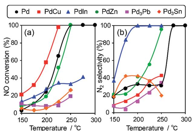
Fig. 2 (a) NO conversion and (b) N<sub>2</sub> selectivity in NO reduction by CO using Pd based catalysts.
