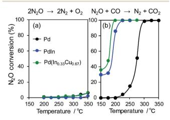
Fig. 7  $\;$  N<sub>2</sub>O (a) decomposition and (b) reduction by CO using Pd, PdIn, and Pd(In $_{0.33}$ Cu $_{0.67}$ ) catalysts.
