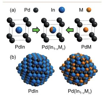
Scheme 1 (a) Concept of the PdIn-based pseudo-binary alloy having a CsCl-type structure with the substitution of In by M. (b) Models of nanoparticulate PdIn and Pd(In $_{1-x}M_x$ ) with a rhombohedral structure surrounded by {110} surfaces. A part of In is replaced by M without modification of Pd.
