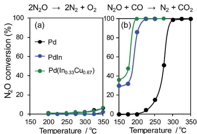
Fig. 7  $N_2O$  (a) decomposition and (b) reduction by CO using Pd, PdIn, and Pd(In<sub>0.33</sub>Cu<sub>0.67</sub>) catalysts.
