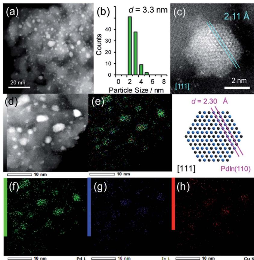
Fig. 3 (a) HAADF-STEM image of Pd–In–Cu/Al<sub>2</sub>O<sub>3</sub> (Pd : In : Cu = 3 : 1 : 2) and (b) size distribution of the nanoparticle. (c) High-resolution STEM image of a single nanoparticle (top) and rhombohedral crystal of PdIn viewed along the [111] direction (bottom). (d) HAADF-STEM image of Pd–In–Cu/Al<sub>2</sub>O<sub>3</sub> and elemental maps of (e) the Pd + In + Cu overlayer, (f) Pd, (g) In, and (h) Cu acquired using EDX.
