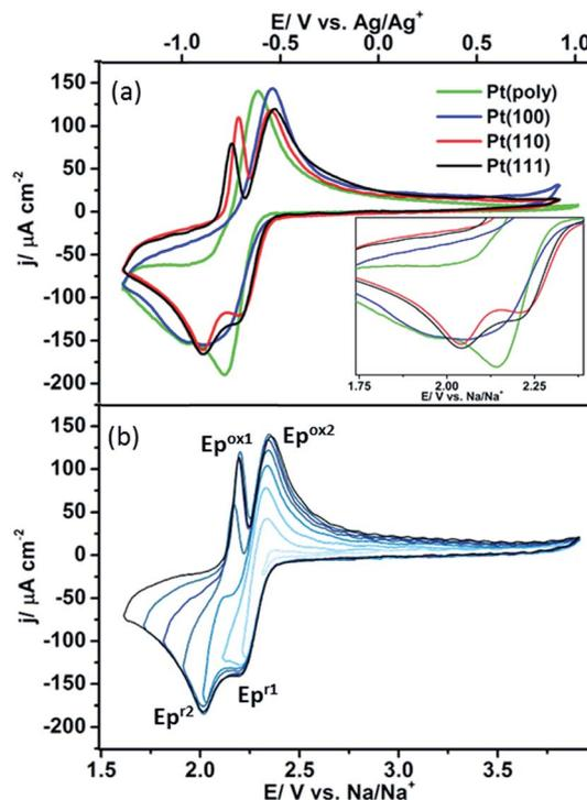
Fig. 2 (a) Cyclic voltammetry of platinum single crystal facets Pt{111}, Pt{110}, Pt{100} and polycrystalline platinum in 0.1 M NaClO<sub>4</sub>, DMSO (O<sub>2</sub> saturated). (Inset) Magnification of the reduction curve demonstrates that surface structure influences the overpotential for the onset of reduction. (b) Potential window opening on Pt{111} showing the association between the two surface redox states at 2.20 and 2.01 V. Sweep rate 50 mV s<sup>-1</sup>.
