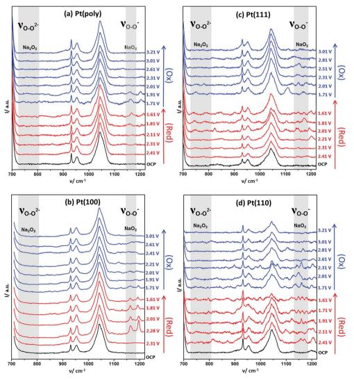
Fig. 3 Full range spectra of EC-SHINERS of 0.1 M NaClO<sub>4</sub> in DMSO on (a) polycrystalline Pt, (b) Pt(100), (c) Pt(111) and (d) Pt(110). All crystal surfaces prepared by flame-annealing and cooling in a CO/water gas stream followed by protection using an irreversibly adsorbed bromide monolayer before the addition of SHINERS nanoparticles. OCP was 2.8 V (key band assignment available in ESI Table S3†).
