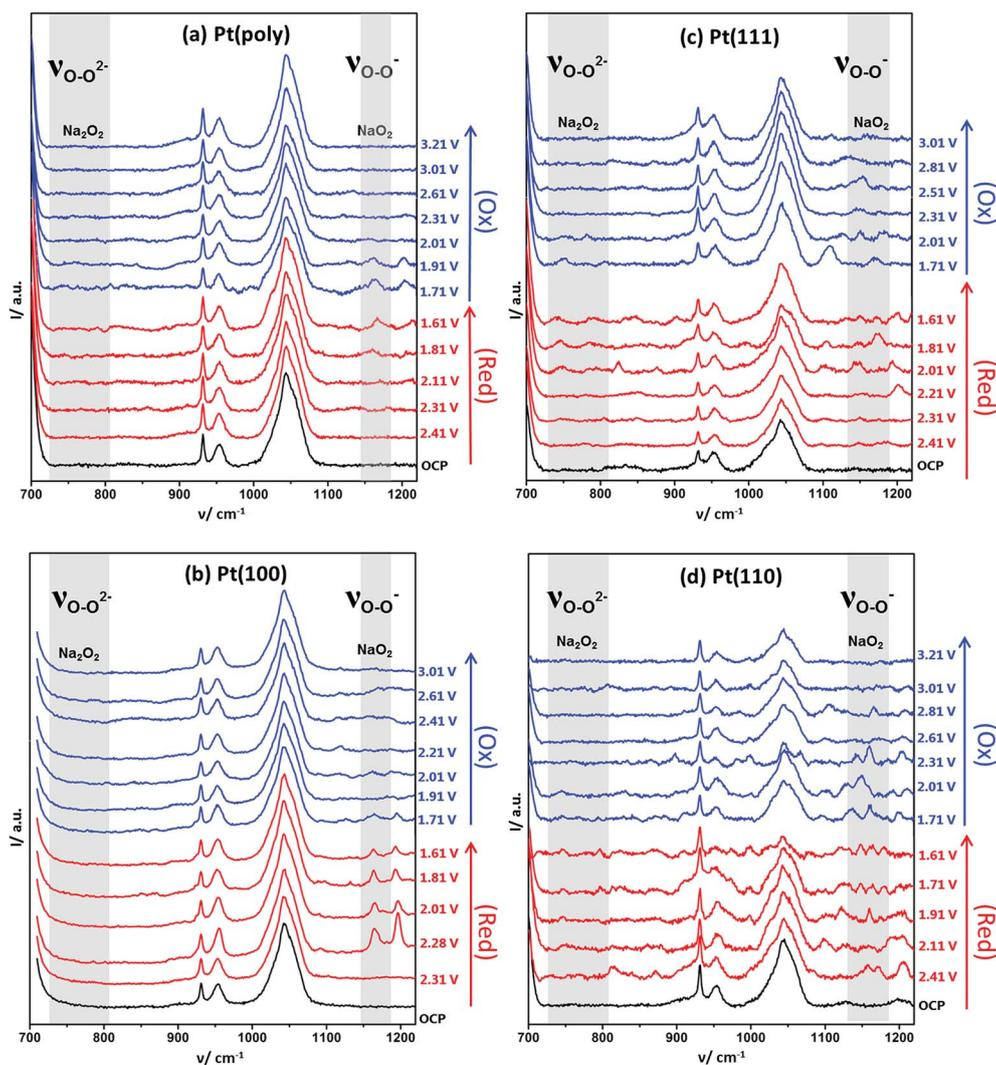
Fig. 3 Full range spectra of EC-SHINERS of 0.1 M  $\text{NaClO}_4$  in DMSO on (a) polycrystalline Pt, (b) Pt{100}, (c) Pt{111} and (d) Pt{110}. All crystal surfaces prepared by flame-annealing and cooling in a CO/water gas stream followed by protection using an irreversibly adsorbed bromide monolayer before the addition of SHINERS nanoparticles. OCP was 2.8 V (key band assignment available in ESI Table S3†).
