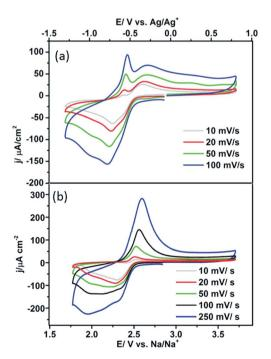
Fig. 6 (a) CVs of 1 M NaClO $_4$  in DMSO (saturated with O $_2$ ) on Pt{111} at different sweep rates, (b) CVs of 0.1 M NaClO $_4$  in DMSO (saturated with O $_2$ ) on Pt{100}, at different sweep rates.
