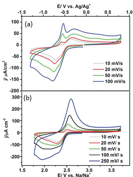
Fig. 6 (a) CVs of 1 M NaClO<sub>4</sub> in DMSO (saturated with O<sub>2</sub>) on Pt{111} at different sweep rates, (b) CVs of 0.1 M NaClO<sub>4</sub> in DMSO (saturated with O<sub>2</sub>) on Pt{100}, at different sweep rates.
