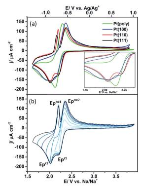
Fig. 2 (a) Cyclic voltammetry of platinum single crystal facets Pt{111}, Pt{110}, Pt{100} and polycrystalline platinum in 0.1 M NaClO<sub>4</sub>, DMSO (O2 saturated). (Inset) Magnification of the reduction curve demonstrates that surface structure influences the overpotential for the onset of reduction. (b) Potential window opening on Pt{111} showing the association between the two surface redox states at 2.20 and 2.01 V. Sweep rate 50 mV s<sup>-1</sup>.
