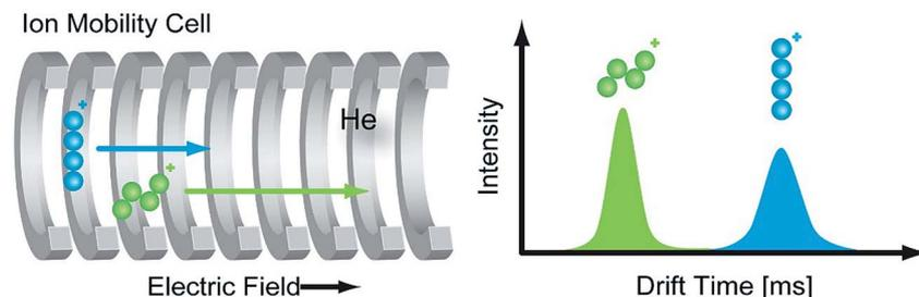
Fig. 2 Principle of ion mobility spectrometry (IMS). In the ion mobility cell ions are separated according to their charge, size, and shape. The IM cell is filled with a neutral buffer gas such as helium or nitrogen. Gas-phase ions travel through the IM cell, guided by a weak electric field, in which larger ions (blue) undergo more collisions with the buffer gas and thus have longer drift times compared to more compact (green) ions.
