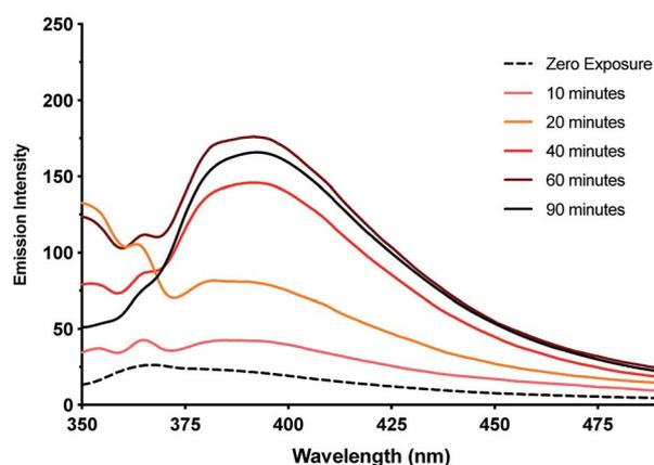
Fig. 11 Emission intensity of metallogel  $1_{\text{MeOH}}$  versus exposure time to UV-light ( $\lambda_{\text{Em}}$ : 395 nm,  $\lambda_{\text{Ex}}$ : 330 nm). Inset emission spectra showing the increase in intensity of the emission band up to 60 minutes exposure.
