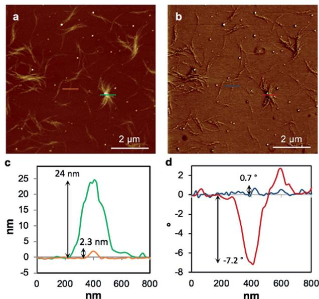
Fig. 8 Tapping mode AFM height image of the 20 times diluted **Xe1** (a), the corresponding EFM phase image (b), line profiles corresponding to the green and orange lines in the AFM height image (c) and a line profile corresponding to the blue and red lines in the EFM phase image (d). The EFM image has been captured at applied DC bias +10 V and a lift height of 30 nm.
