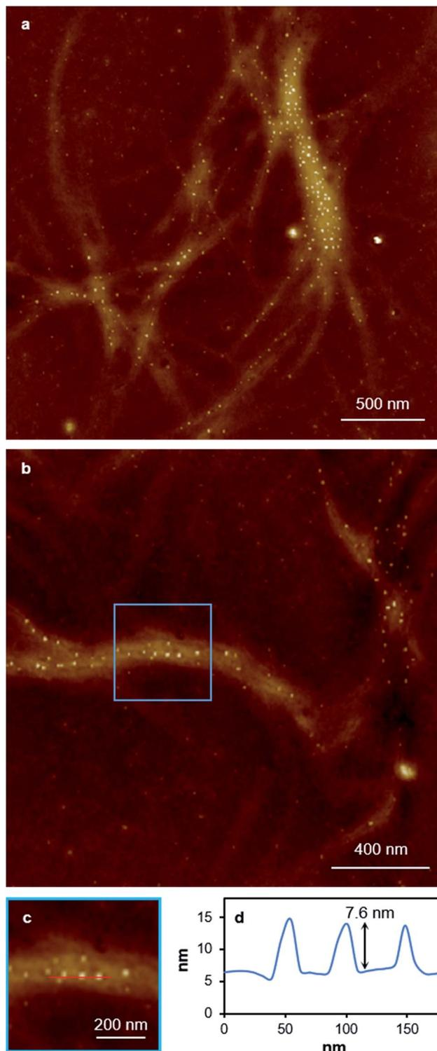
Fig. 10 AFM height images of a 20-times diluted sample of xerogel **Xe1**. Large scan range images (a) and zoom-in (b) showing Ag-particles embedded in gel fibres. Zoom-in area (c) showing the location of the line profile, and (d) a line profile corresponding to the red line in the image (c). The line profile along a single fibre in the AFM image (c) shows nanoparticles that protrude from the underlying fibre by  $\sim 7.6$  nm with an estimated overall diameter of  $\sim 14$  nm.
