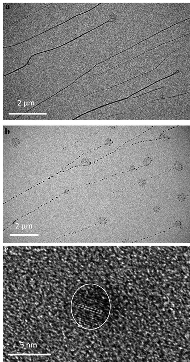
Fig. 12 TEM bright field images of gel before and after illumination. (a) Homogeneous fibres in keeping with the regular metallo-array in **1** and (b) after illumination showing the formation of electron-dense nanoparticles along the fibre axis. (c) HR-TEM image of a silver particle (dia. 4.3 nm) with lattice fringe spacing  $0.25 \text{ nm} \pm 0.02$  corresponding to the interplanar distances of (111).
