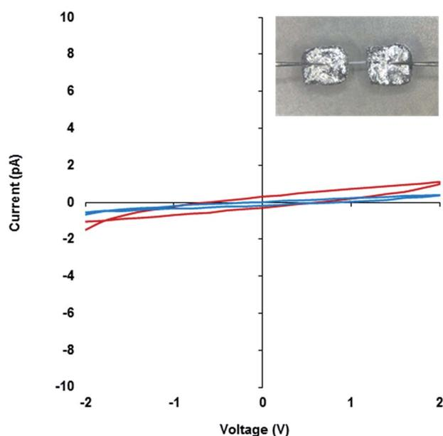
Fig. 7 *I*–*V* curves of the  $1_{\text{MeOH}}$  xerogel (red) and crystal of **1** (blue). Inset, an optical microscope image of a single crystal of **1** connected to probe station tips through Ga–In eutectic along the crystallographic *c*-axis.
