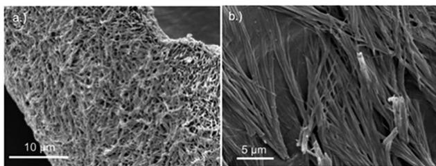
Fig. 2 SEM images of bis(cytidine)-silver(I) xerogel, **1**<sub>MeOH</sub>. (a) Xerogel showing the entangled porous polymer matrix. (b) Micrograph showing bundling of fibres.
