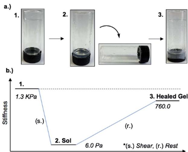
Fig. 6 (a) Optical images of the material through application or removal of shear. Inversion test showing the thixotropic nature of  $1_{\text{MeOH}}$  ((1) gel, (2) sol and (3) healed gel). (b) A generalised schematic representing the stiffness of the gel through a thixotropic cycle.
