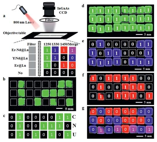
Fig. 3 (a) Scheme of an invisible SWIR logical code, and "OR" and "AND" logical operations with optical filters; (b) SWIR image collected by a 1250 filter of a  $3 \times 8$  array containing Er@Lu, Y:Nd@Lu and Er-Nd@Lu and the corresponding SWIR logical code (c); SWIR images collected by a 1250 filter (d), 1330 filter (e) and 1450 filter (f) of a  $3 \times 8$  array containing Er@Lu, Y:Nd@Lu and Er-Nd@Lu and an "AND" logical operation (g) between images e and f.
