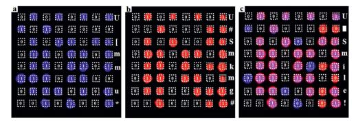
Fig. 4 Invisible SWIR logical code for the information ("U Smile!") encryption experiment; SWIR pseudo-color images, and logical coding and corresponding decoding information of single Nd<sup>3+</sup> emission (a), single Er<sup>3+</sup> emission (b) and "AND" logical operation (c).
