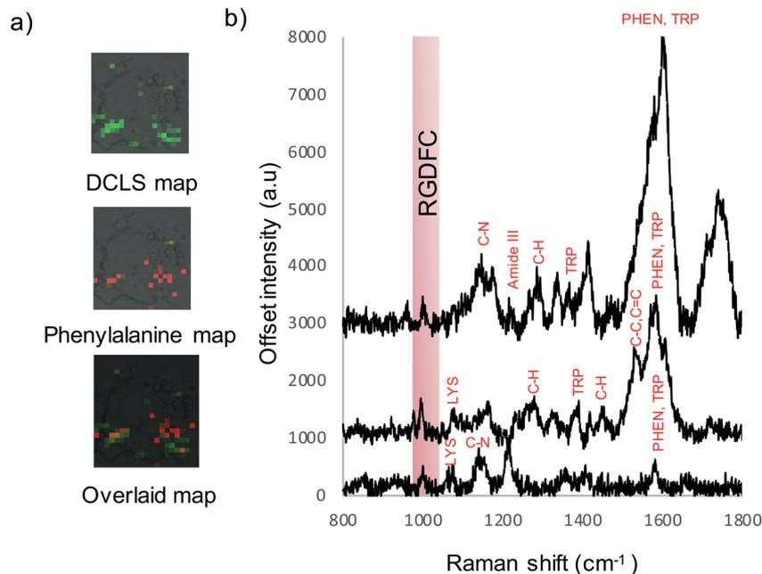
Fig. 5 (a) False color images created using DCLS analysis, RGDFC peak at  $1000\text{ cm}^{-1}$  analysis and the two overlaid indicating areas of overlap. (b) Selected spectra from map indicating RGDFC peaks and peaks of the bound  $\alpha_v\beta_3$  integrin spectrum. Cells were mapped using a  $50\times$  microscope objective,  $1 \times 1\ \mu\text{m}$  step size,  $633\text{ nm}$  laser excitation with a laser power of  $4\text{ mW}$ , scanning between  $800\text{--}2000\text{ cm}^{-1}$ .
