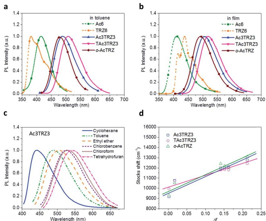
Fig. 3 Steady-state photophysical properties of the TSCT-HABs. PL spectra of the TSCT-HABs in toluene ( $10^{-5}$  mol  $L^{-1}$ ) (a) and in the film state (b), PL spectra of Ac3TRZ3 in solvents with different polarity (c), and the linear correlation of orientation polarization ( $\Delta f$ ) of the solvent with the Stokes shift for the TSCT-HABs (d) (see Table S1† for data).
