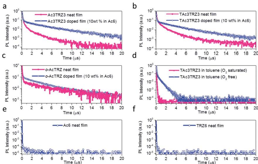
Fig. 4 Transient PL decay of the TSCT-HABs. PL decay curves of the Ac3TRZ3, TAc3TRZ3 and *o*-AcTRZ in neat or doped films (a–c), TAc3TRZ3 in  $N_2$  or  $O_2$  saturated toluene ( $10^{-5}$  mol  $L^{-1}$ ) (d), and the Ac6 and TRZ6 neat films (e and f).
