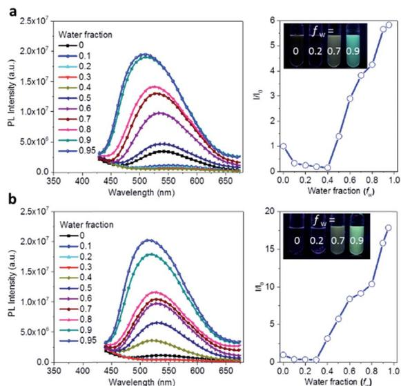
Fig. 5 Aggregation-induced emission effect of the TSCT-HABs. PL spectra and the relative emission intensity of Ac3TRZ3 (a) and TAc3TRZ3 (b) in THF/water mixed solvents at a concentration of  $1 \times 10^{-5}$  mol L $^{-1}$ ; inset: PL images with different water fractions ( $f_w$ ) under UV light (365 nm).
