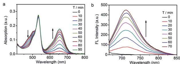
Fig. 1 Time-dependent (a) absorption and (b) emission spectral changes of TNP-SO (5 μM) in the presence of 100 μM NaHS under physiological conditions (CH<sub>3</sub>CN/PBS, 1 : 1, v/v, 20 mM, pH 7.4, and room temperature). λ<sub>ex</sub> = 640 nm.
