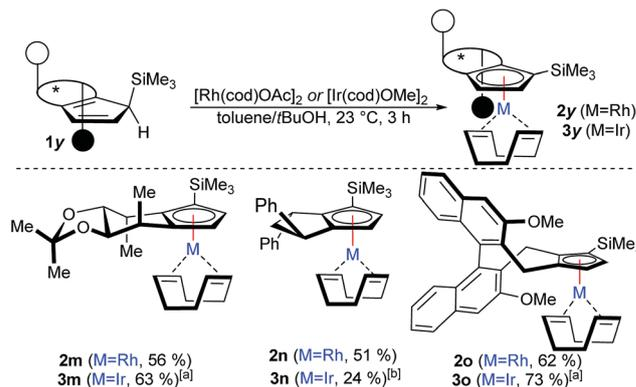
Scheme 4 Diastereoselective complexation with TMS-Cp<sup>x</sup> ligands: 0.1 mmol **1y**, 0.06 mmol [Rh(cod)OAc]<sub>2</sub>, toluene/*t*BuOH, at 23 °C for 3 h. (a) With [Ir(cod)OMe]<sub>2</sub> (b) with [Ir(cod)OAc]<sub>2</sub>.
