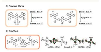
Fig. 1 (A) Chemical structures and electronic properties of previously reported SWIR AIE fluorogens (TQ-BPN and TB1). (B) Chemical structure, frontier molecular orbital amplitude plots and electronic properties of the BBTD-based NIR-II AIE fluorogen. All molecular fluorophores were calculated using B3LYP/6-31G (d, p).
