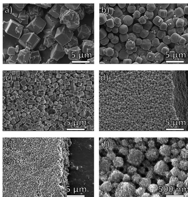
Fig. 5 SEM images of polyIRMOF-1 prepared from polymer ligands: (a) pbdc-8a; (b) pbdc-8a-PEG<sub>2000</sub>-2%; (c) pbdc-8a-PEG<sub>4000</sub>-1%; (d) pbdc-8a-PEG<sub>2000</sub>-20%; (e and f) pbdc-8a-PEG<sub>4000</sub>-10%.
