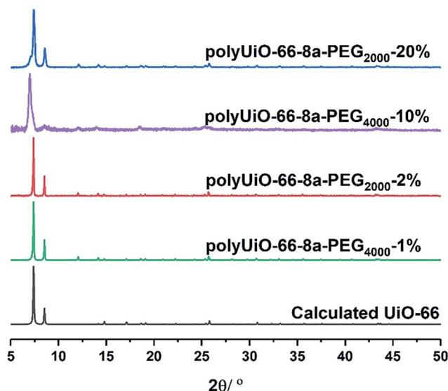
**Fig. 1** PXRD patterns of polyUiO-66 prepared from pbdc-8a-PEG<sub>*M<sub>n</sub>*</sub>-*x*% block copolymers.
