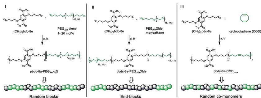
**Scheme 1** Synthesis of three types of polymer ligands used in this work: (i) random AB PEG block copolymer ligand (pbdc-8a-PEG<sub>M<sub>n</sub></sub>-x%); (ii) capped AB<sub>2</sub> PEG block copolymer ligand (pbdc-8a-PEG<sub>M<sub>n</sub></sub>OMe); (iii) random AB COD block copolymer ligand (pbdc-8a-COD<sub>m:n</sub>). Reagents and conditions: (a) G2 catalyst, CH<sub>2</sub>Cl<sub>2</sub>, 50 °C, 5 h; (b) KOH, THF/H<sub>2</sub>O, 40 °C, 12 h.
