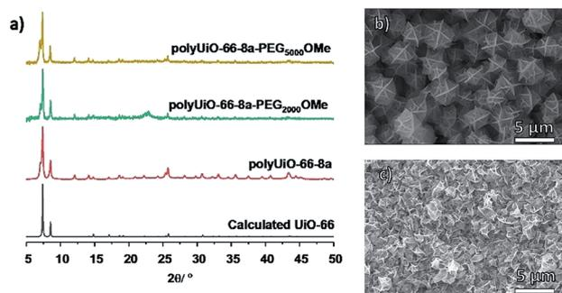
Fig. 3 (a) PXRD patterns of polyUiO-66 prepared from purified pbdc-8a-PEG<sub>*M<sub>n</sub>*</sub>OME. SEM images of polyUiO-66 prepared from: (b) pbdc-8a-PEG<sub>2000</sub>OME and (c) pbdc-8a-PEG<sub>5000</sub>OME.
