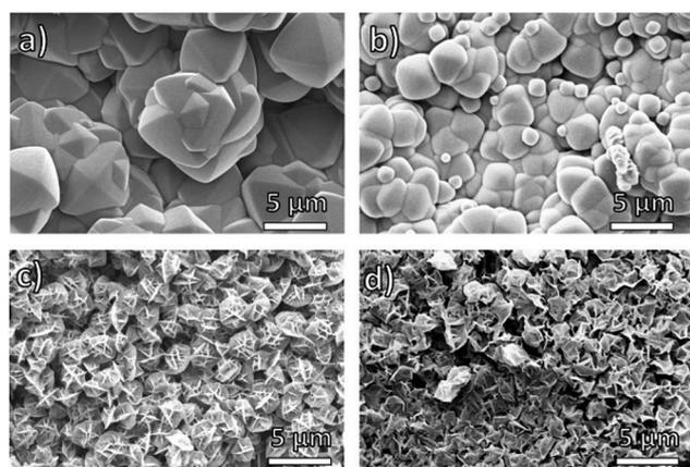
Fig. 2 SEM images of polyUiO-66 prepared from block copolymer ligands: (a) pbdc-8a-PEG<sub>2000</sub>-2%; (b) pbdc-8a-PEG<sub>4000</sub>-1%; (c) pbdc-8a-PEG<sub>2000</sub>-20%; (d) pbdc-8a-PEG<sub>4000</sub>-10%.
