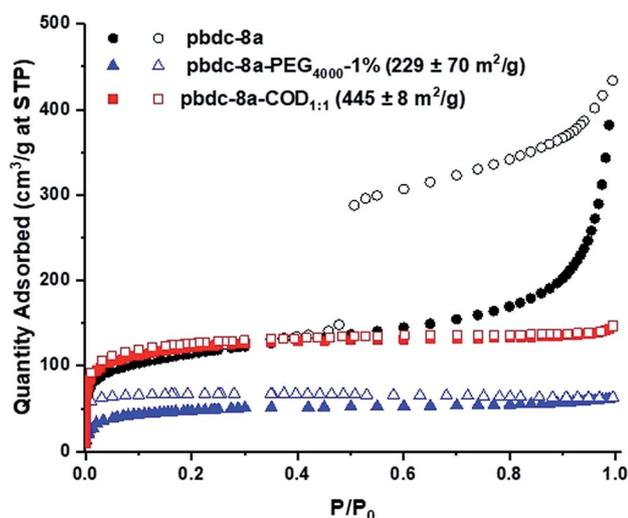
Fig. 4 Representative N<sub>2</sub> isotherms of block-polyUiO-66 prepared from various block copolymer ligands that result in intergrown octahedra. The BET surface areas are included in parentheses. polyUiO-66 prepared from homopolymer pbdc-8a is included for comparison. Closed and open symbols represent the adsorption and desorption processes, respectively.
