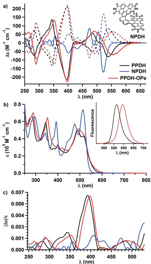
Fig. 2 (a) ECD, (b) UV-visible absorbance, and (c) *g*-factors of PPDH, PPDH-OPe, and NPDH in THF (10  $\mu\text{M}$ , 1 cm path length). (Inset of b) Normalized fluorescence intensities of PPDH and PPDH-OPe in cyclohexane (3  $\mu\text{M}$ ,  $\lambda_{\text{ex}} = 410 \text{ nm}$ ;  $\Phi_f = 41\%$  and 15% for PPDH and PPDH-OPe, respectively). For NPDH, R =  $\text{CH}(\text{C}_5\text{H}_{11})_2$ .
