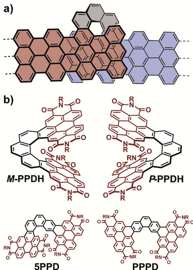
Fig. 1 (a) The fusion of two armchair nanographenes with phenanthrene provides a  $\pi$ -extended bilayer helicene. (b) Fusion with two PDI subunits *via* oxidative photocyclization at elevated temperatures overwhelmingly favors the formation of PPDH over its isomers, 5PPD and PPPD.
