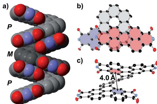
Fig. 3 Structure of PPDH from SCXRD. Free solvent, the  $\text{CH}(\text{C}_5\text{H}_{11})_2$  chains, and hydrogen atoms have been hidden to provide an unobstructed view of the aryl surface. Thermal ellipsoids are set at 30% probability. (a) The racemate assembles as heterochiral columns in the solid state. Extensive intramolecular overlap between the PDI subunits (b) distorts their perylene cores into shallow bowls (c).
