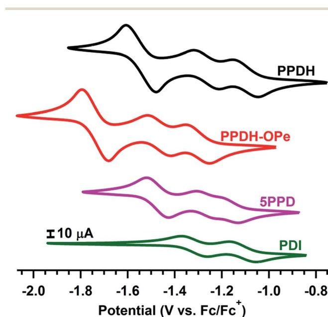
Fig. 4 Cyclic voltammograms of **PPDH**, **PPDH-OPe**, **5PPD**, and monomeric PDI (1 mM, 50 mV s<sup>−1</sup> scan rate) in Ar-sparged DCM with 0.1 M [Bu<sub>4</sub>N][PF<sub>6</sub>] as the supporting electrolyte. For all species, R = CH(C<sub>5</sub>H<sub>11</sub>)<sub>2</sub>.
