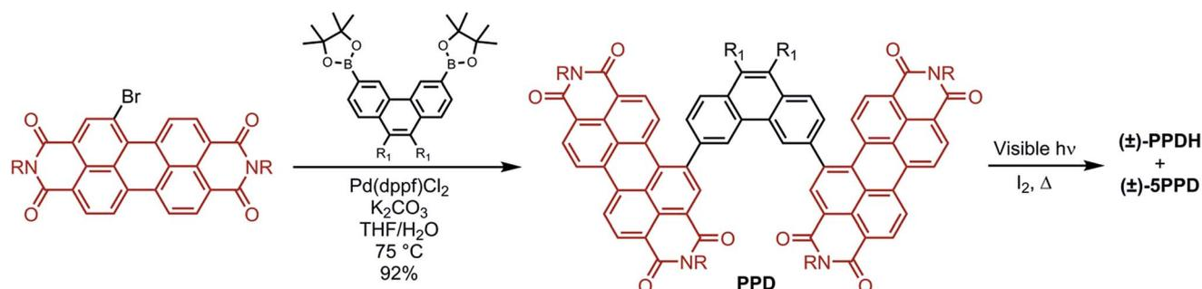
Scheme 1 Two-step synthesis of PPDH from brominated PDI [R = CH(C<sub>5</sub>H<sub>11</sub>)<sub>2</sub>].
