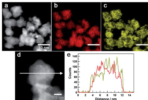
Fig. 3 Scanning transmission electron microscopy images of  $\text{Au}_{0.5}\text{Ir}_{0.5}$  NPs. (a) a HAADF-STEM image. (b), (c) Au-M and Ir-M STEM-EDX maps (red, Au; yellow, Ir). (e) Compositional line profiles of Au (red) and Ir (dark yellow) for the  $\text{Au}_{0.5}\text{Ir}_{0.5}$  nanoparticle recorded along the arrow shown in (d) the HAADF-STEM image.
