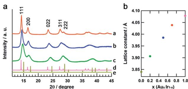
Fig. 4 X-ray diffraction analysis of  $\text{Au}_x\text{Ir}_{1-x}$  NPs. (a) Powder XRD patterns of a;  $\text{Au}_{0.7}\text{Ir}_{0.3}$  NPs, b;  $\text{Au}_{0.5}\text{Ir}_{0.5}$  NPs, c;  $\text{Au}_{0.2}\text{Ir}_{0.8}$  NPs, d; Au and e; Ir powders. (b) A plot of the changes in the lattice constants versus the metal composition.
