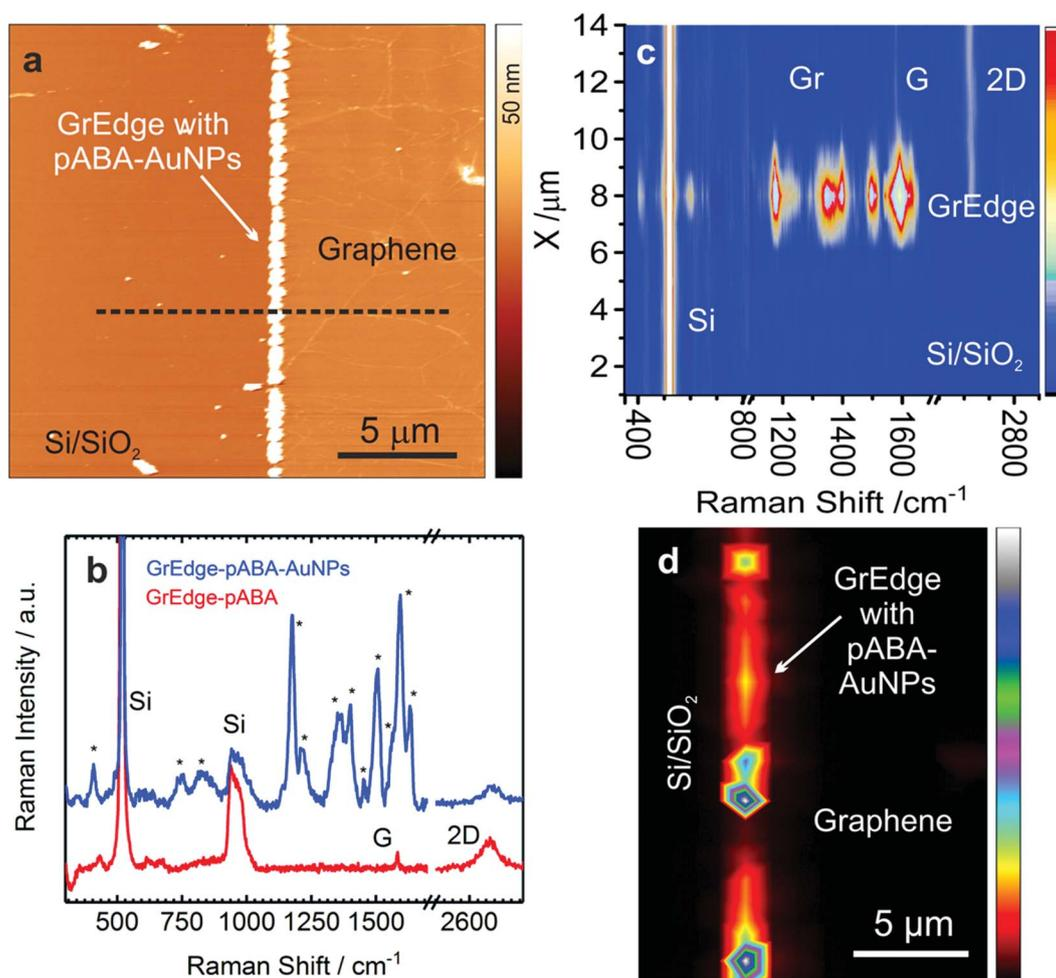
Fig. 3 (a) AFM image of a typical GrEdge functionalized with poly(aminobenzylamine) (pABA) and AuNPs, referred to as GrEdge-pABA-AuNPs. (b) Comparison of the Raman spectra at GrEdge-pABA (red curve) and GrEdge-pABA-AuNPs (blue curve). (c) Raman map along the line shown in (a). (d) Map of the C-N stretching mode ( $1358\text{ cm}^{-1}$ ) of the same region as in (a) ( $\lambda_{\text{ex}}$ :  $633\text{ nm}$ ,  $3.4\text{ mW}$ ,  $2 \times 1\text{ s}$ ).
