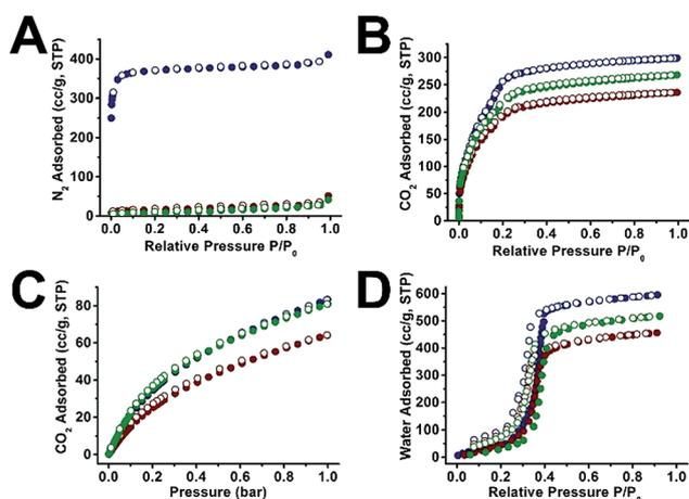
Fig. 4 N<sub>2</sub> sorption isotherms at 77 K (A), CO<sub>2</sub> sorption isotherms at 195 K (B) and 273 K (C), and water vapor sorption isotherms at 298 K (D) of UiO-66 (navy), UiO-66@xPS (red) and UiO-66@xPBA (green). UiO-66@xPS and UiO-66@xPBA isotherms were normalized by subtracting the mass of the polymer (Table S5†).
