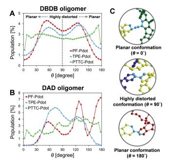
Fig. 4 Distributions of the torsional angle between (A) the donor and bridge on the DBDB oligomers, and between (B) the donor and acceptor on the DAD oligomers; (C) the representative planar conformations ( $\theta \sim 0^{\circ}$  or  $\sim 180^{\circ}$ ) and highly distorted conformation ( $\theta \sim 90^{\circ}$ ), where the torsional angles are marked in light blue color and hydrogen atoms are not shown for clarity.
