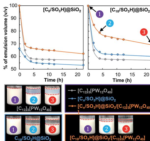
Fig. 5 Evolution of the emulsion volume fraction (S.D. = 2%) as a function of the storage time at 60 °C for the  $[C_n/SO_3H]@SiO_2$  and  $[C_{12}]_3[PW_{12}O_{40}]$  emulsions (1/1 v/v) stabilized by  $[C_n/SO_3H]@SiO_2$  and  $[C_{12}]_3[PW_{12}O_{40}]$  NPs or a mixture of both NPs (3.6 wt%,  $\phi = 0.5$ , 11 500 rpm). The insets show the W/O emulsions stabilized by  $[C_{18}/SO_3H]@SiO_2$  and/or  $[C_{12}]_3[PW_{12}O_{40}]$  NPs.
