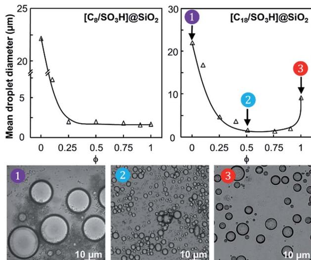
Fig. 3 Evolution of the droplet size (S.D. = 10%) as a function of the  $[C_n/SO_3H]@SiO_2$  mass fraction ( $\phi$ ) for water/toluene Pickering emulsions (1/1 v/v) stabilized by  $[C_n/SO_3H]@SiO_2$  and  $[C_{12}]_3[PW_{12}O_{40}]$  NPs (3.6 wt%, 11 500 rpm). The insets present the micrographs of the W/O emulsions.
