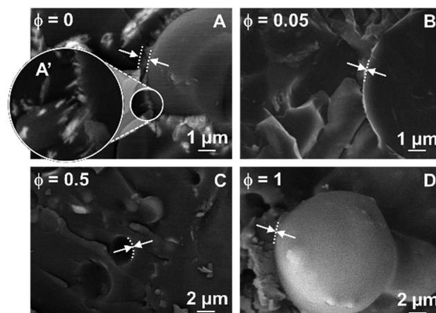
Fig. 7 Cryo-SEM micrographs of water/toluene emulsions (1/1 v/v) as a function of the  $[C_{18}/SO_3H]@SiO_2$  mass fraction ( $\phi$ ) for  $[C_{18}/SO_3H]@SiO_2/[C_{12}]_3[PW_{12}O_{40}]$  mixtures (3.6 wt%, 11 500 rpm). The white arrows and the dashed lines indicate the thickness of the NPs layer.
