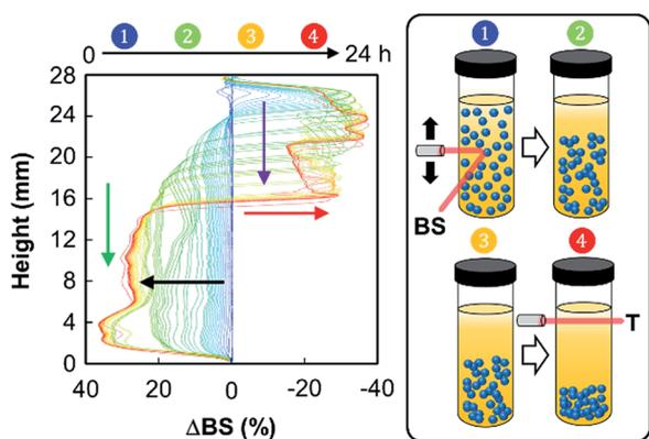
Fig. 6 Variation of backscattering at 60 °C ( $\Delta BS$ ) versus sample height and time of  $[C_{18}/SO_3H]@SiO_2/[C_{12}]_3[PW_{12}O_{40}]$  mixtures (3.6 wt%,  $\phi = 0.5$ , 11 500 rpm) from 0 (blue curve) to 24 h (red curve). The inset shows a representation of the time-evolution of the clarification/sedimentation process (T = transmitted light and BS = backscattered light) of the emulsion.
