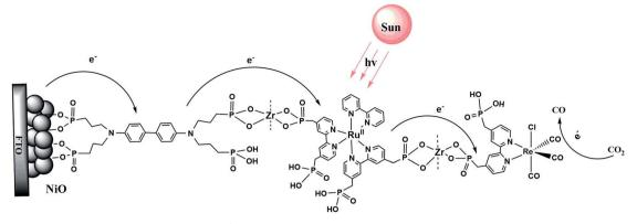
Scheme 1 Structure of the assembly NiO|-DA-RuCP<sub>2</sub><sup>2+</sup>-Re(i) on a mesoporous NiO electrode
