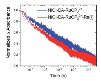
Fig. 6 Normalized transient absorption changes measured at 530 nm after pulsed 488 nm excitation of NiO|-DA-RuCP $_2$ <sup>2+</sup> (blue) and NiO|-DA-RuCP $_2$ <sup>2+</sup>-Re(i) (red) at -0.8 V vs. NHE in argon-saturated 0.1 M LiClO $_4$  acetonitrile solution.
