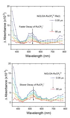
Fig. 5 Nanosecond transient absorption difference spectra measured after pulsed 488 nm light excitation of NiO|-DA-RuCP $_2^{2+}$ -Re(i) (top) and NiO|-DA-RuCP $_2^{2+}$  (bottom) in 0.1 M LiClO $_4$  acetonitrile with -0.8 V vs. NHE applied potential under argon.
