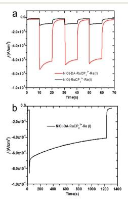
Fig. 3 (a) Photocurrent density *versus* time (j-t) plots for NiO assemblies with three 10 s dark–light (one sun illumination) cycles with an applied bias of -0.54 V vs. NHE in 0.1 M in LiClO<sub>4</sub> acetonitrile under 1 atm CO<sub>2</sub>. (b) Photocurrent response of NiO|-DA-RuCP<sub>2</sub><sup>2+</sup>-Re(i), over a 20 min period under the same conditions as described for (a).
