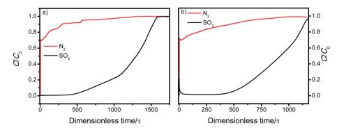
Fig. 3 Dimensionless breakthrough curve of 0.25% SO<sub>2</sub> (2500 ppm) diluted in He/N<sub>2</sub> under (a) dry and (b) wet conditions through a fixed-bed packed with MFM-305 at 298 K and 1 bar.
