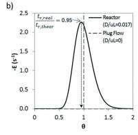
Fig. 5 a) Example of an RTD curve during step tracer experiments to estimate gas dispersion in the drop tube apparatus (T = 750 °C, inlet gas flow of 2.7 Nm3 h<sup>-1</sup>). System I includes the drop tube, analyzer and connecting line and system II refers to the pipeline downstream of the reactor and the analyzer; b) deviation from ideal plug flow for a pulse input.
