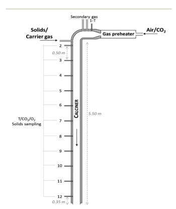
Fig. 2 Scheme of the drop tube reactor used in this work for the determination of calcination kinetics of cement raw meals.
