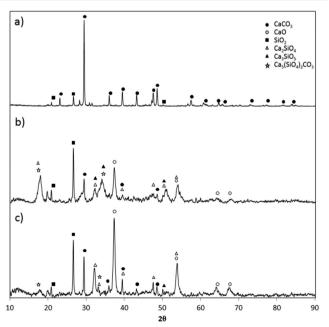
Fig. 4 X-Ray diffractograms of fresh and calcined Vernasca raw meal: a) fresh sample, b) calcined sample (at 840 °C in air for 0.5 s), and c) calcined sample (at 950 °C in air for 0.3 s).
