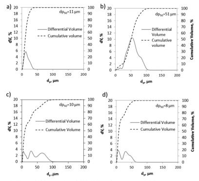
Fig. 3 Particle size distribution of different CaCO<sub>3</sub> materials: a) CP3, b) CP1, c) Vernasca, and d) Calcare.
