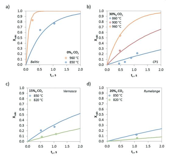
Fig. 8 Effect of temperature on the calcination conversion for CaCO<sub>3</sub> materials of different origins and compositions. a) Belitic (mixture of limestone and marl), b) CP1 (limestone), c) Vernasca (mixture of limestone and marl), and d) Rumelange (mixture of limestone and marl). Solid lines correspond to model predictions.
