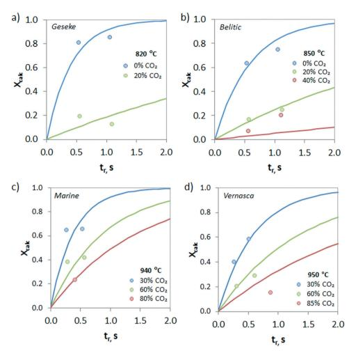
Fig. 9 Effect of the concentration of  $CO_2$  in the gas phase on the calcination conversion for  $CaCO_3$  materials of different origins and compositions. a) Geseke (marl), b) Belitic (mixture of limestone and marl), c) Marine (marl), and d) Vernasca (mixture of limestone and marl). Solid lines correspond to model predictions.
