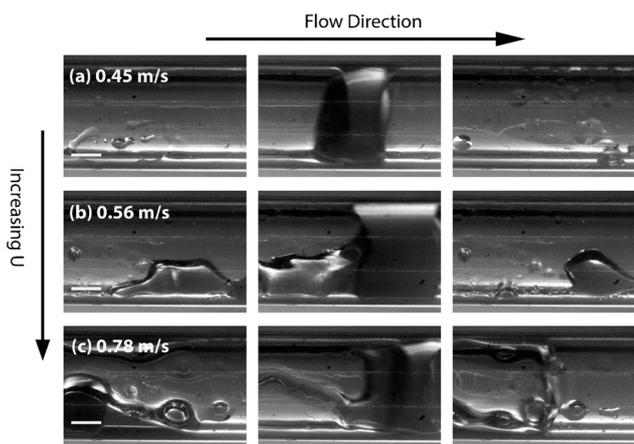
**Fig. 4** (a)–(c) High-speed stereomicroscope images at higher flow velocities in 2 m long 3.2 mm ID PTFE channel, highlighting the extent of droplet breakup with increasing flow speed.  $Q_{Org} = 0.1$  mL  $min^{-1}$ ,  $Q_{Aq} = 0.3$  mL  $min^{-1}$ ,  $Q_{Gas} = 115$  mL  $min^{-1}$ , 120 mL  $min^{-1}$  and 146 mL  $min^{-1}$  respectively. All scale bars represent 1 mm.
