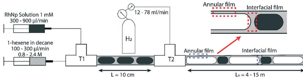
**Fig. 1** Schematic representation of the triphasic gas-liquid-liquid segmented flow experimental setup. The interfacial film is the thin organic segment separating the bubble and aqueous droplet caps, whereas the annular film is the organic lubricating film surrounding all gas bubbles.
