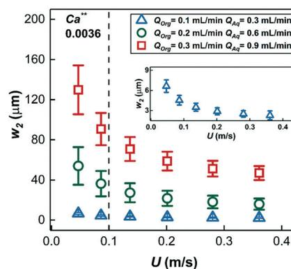
**Fig. 8** The thickness of the annular film around the gas bubbles estimated by fitting the mathematical model of eqn (3) at different volumetric liquid flow rates and bubble speeds. Insert shows a magnified view of the thickness of the annular film for  $Q_{\text{Org}} = 0.1 \text{ mL min}^{-1}$ ,  $Q_{\text{Aq}} = 0.3 \text{ mL min}^{-1}$ . (for  $Ca^{**}$  see ESI† section 1).
