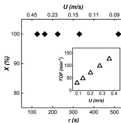
Fig. 10 1-Hexene conversion ( $X$ ) versus bubble residence time ( $\tau$ ) in scaled-up mesoreactor. Insert shows the turnover frequency of the reactor at different flow velocities. Turnover frequency is defined as number of moles of 1-hexene converted to product per number of moles of catalyst per unit time.
