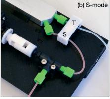
Fig. 4 Photographs showing the two operating modes for the separator, achieved via a simple reconfiguration of the outlet tubing. The motorised valve is always connected to the under-pressured outlet, so the T-mode configuration (a) is used when the T-channel is underpressured, and the S-mode configuration (b) is used when the S-channel is under-pressured. Note, DCM in S-channel has been dyed with Sudan orange.
