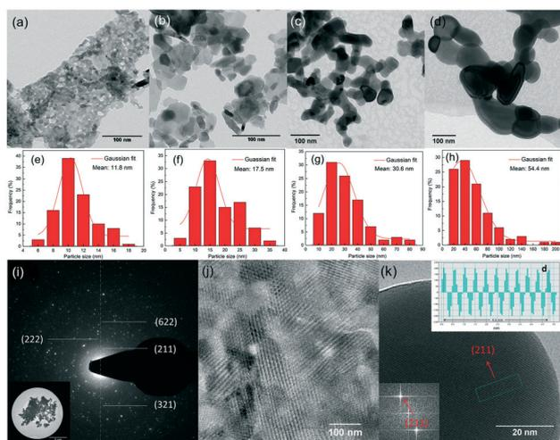
Fig. 4 TEM images of 5%  $\text{Eu}^{3+}$  doped yttria nanophosphors with heat treatment at (a) 600 °C, (b) 800 °C, (c) 1000 °C and (d) 1200 °C; (e–h) the corresponding size distributions; (i–k) SAED pattern and HRTEM images of the 5%  $\text{Eu}^{3+}$  doped yttria nanophosphors obtained at 1200 °C.
