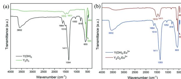
Fig. 3 (a) FTIR spectra of the dried  $Y(OH)_3$  and  $Y_2O_3$  nanoparticles annealed at 600 °C; (b) FTIR spectra of the dried  $Y(OH)_3:5\%Eu^{3+}$  and  $Y_2O_3:5\%Eu^{3+}$  nanoparticles annealed at 600 °C.
