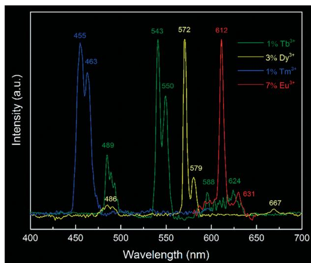
Fig. 7 Typical photoluminescence emission spectra of  $\text{Ln}^{3+}$  doped yttria nanophosphors: 1%  $\text{Tb}^{3+}$  doping, excited at 307 nm; 3%  $\text{Dy}^{3+}$  doping, excited at 355 nm; 1%  $\text{Tm}^{3+}$  doping, excited at 355 nm and 7%  $\text{Eu}^{3+}$  doping, excited at 248 nm. All spectra were normalized at the same level. The measuring conditions were referenced to reported values in the literature.<sup>41</sup>
