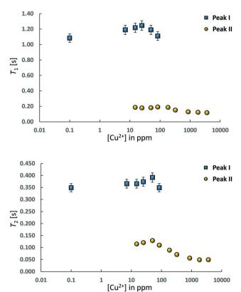
Fig. 3  $T_1$  and  $T_2$  values for 1-octene in CuSO<sub>4</sub>/Al<sub>2</sub>O<sub>3</sub> samples at different concentration of CuSO<sub>4</sub>, expressed as [Cu<sup>2+</sup>]. Peak I is associated to 1-octene interacting with Al<sub>2</sub>O<sub>3</sub> whilst peak II is that of 1-octene interacting with CuSO<sub>4</sub>. The paramagnetic nature of Cu<sup>2+</sup> ions leads to much smaller values of  $T_1$  and  $T_2$  NMR relaxation times of peak II.
