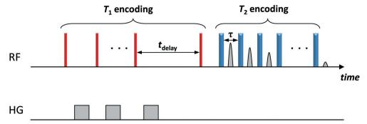
Fig. 1 Two-dimensional  $T_1$ - $T_2$  NMR pulse sequence. The thin (red) and thick (blue) vertical bars represent 90° and 180° radiofrequency (RF) pulses, respectively.  $T_1$  relaxation is encoded in the variable time  $t_{\text{delay}}$ .  $T_2$  relaxation is encoded in the train of n 180° pulses. A single data point is acquired at the centre of each echo time, r. The grey bars (HG) represent homospoil magnetic field gradients.
