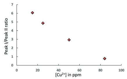
Fig. 4 Area ratio of peak I, associated to Al<sub>2</sub>O<sub>3</sub>, over peak II, associated to CuSO<sub>4</sub>, as a function of [Cu<sup>2+</sup>] for samples where both peaks are present in the  $T_1$ - $T_2$  NMR correlation maps.
