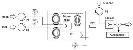
Fig. 1 Microreactor setup for kinetic investigations, including syringe pumps (P1, P2, P3), the reactor unit (R1), and a back pressure regulator (BPR).
