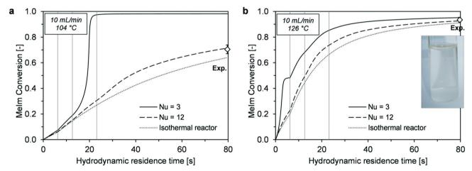
Fig. 12 Simulated conversion profiles for different Nusselt numbers with isothermal reactor operation and experimentally determined conversions at the plate reactor outlet: a)  $T_{\rm w}=104\,^{\circ}{\rm C}$ ,  $\dot{V}_{\rm ges}=10\,$  mL min<sup>-1</sup>; and b)  $T_{\rm w}=126\,^{\circ}{\rm C}$ ,  $\dot{V}_{\rm ges}=10\,$  mL min<sup>-1</sup>; sample of the nearly colorless product obtained at the reactor outlet.
