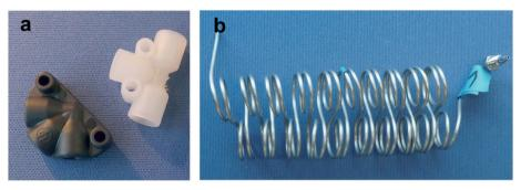
Fig. 2 a) T-Mixer and arrowhead mixer. b) Coiled capillary reactor.
