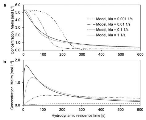
Fig. 7 Simulations of the Melm concentration in the reaction phase (a) and product phase (b) to demonstrate the influence of  $k_{\parallel}a$  on the reaction rate.
