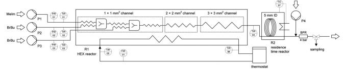
Fig. 3 Reactor setup for scale-up experiments in a millistructured aluminum plate reactor (R1) and an additional residence time reactor (R2), including syringe pumps (P1, P2, P3), and a back pressure regulator (BPR).
