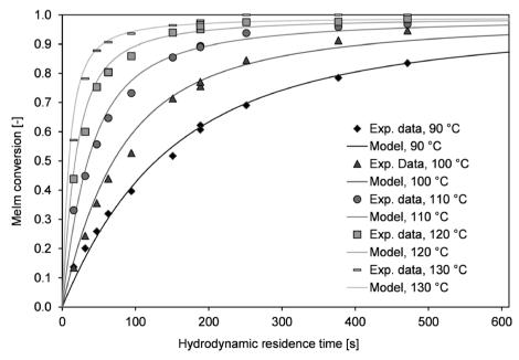
Fig. 8 Experimental (Exp.) data determined with both capillary reactors (lengths of 2 m and 8 m), and curve fitting results based on the described reaction model. Comparison of different reactor temperatures at a reactant molar ratio of  $c_{\text{MeIm},0}/c_{\text{BrBu},0}=1.01$ .
