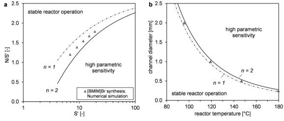
Fig. 9 Reactor stability diagrams in dimensionless form (a) and with practical operating parameters (b). Comparison of simulated results (twophase model) with the empirical correlation based on Baerns and Renken<sup>31</sup> for first- and second-order reactions (single-phase model).
