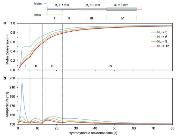
Fig. 11 Simulation of conversion (a) and temperature (b) for [BMIM]Br synthesis in the aluminum plate reactor for  $T_w = 130$  °C and  $\dot{V}_{\rm qes} = 10$  mL min<sup>-1</sup> with different Nusselt numbers. The multi-injection reactor principle was applied with two BrBu injections at the same flow rate.
