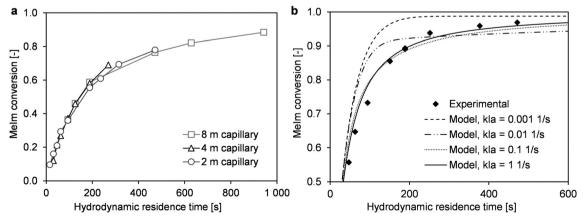
Fig. 6 a) Comparison of experimentally determined conversions for reactor capillaries with different lengths (i.d. 1 mm, T = 90 °C). b) Simulated conversion results for different  $k_{\rm l}a$  values compared with the experimental conversion results ( $T=110\,^{\circ}{\rm C}$ ,  $c_{\rm Melm,0}/c_{\rm BrBu,0}=1$ ).
