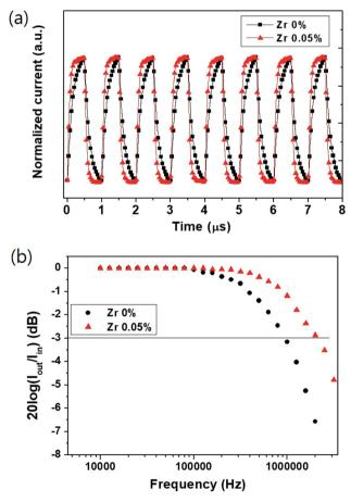
Fig. 4 Dynamic characteristics of photocurrent response times using a laser diode at a light intensity of 650  $\mu$ W cm<sup>-2</sup> at 525 nm. (a) Photocurrent response time under -0.1 V at a pulsed frequency of 1 MHz. (b) Cut-off frequency for the perovskite photodetector under -0.1 V.
