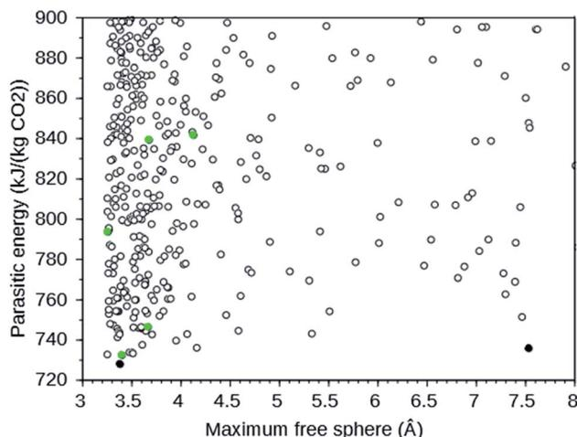
Fig. 1 Parasitic energy *versus* maximum free sphere diameter of IZA (green) and theoretical (black) zeolite frameworks screened by ref. 7. The plot is cut off at a parasitic energy of 900 kJ (kg CO<sub>2</sub>)<sup>-1</sup> and a maximum free sphere of 8 Å. The filled circles are the target frameworks we selected. The data were downloaded from ref. 9.
