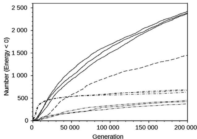
Fig. 2 Number of designed molecules with a stabilization energy below  $0 \text{ kJ (mol Si)}^{-1}$  as a function of the number of molecules generated in the course of the *de novo* design runs on the DAC framework using the MS10 shelf (solid line), the MS15 shelf (dashed line), the MS05 shelf (dot-dashed line), and on the GIS framework with the MS10 shelf (double-dot-dashed line).
