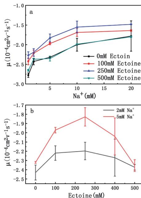
Fig. 2 (a) EM of DNA *versus* the concentration of  $\text{Na}^+$  with 0 mM, 100 mM, 250 mM and 500 mM ectoine respectively. (b) EM of DNA *versus* the concentration of ectoine with 2 mM and 5 mM  $\text{Na}^+$  respectively in solution. 10 mM Tris (pH = 7.5) buffer is used, and the concentration of DNA is  $1 \text{ ng } \mu\text{L}^{-1}$ . The error bars represent the corrected sample standard deviation.
