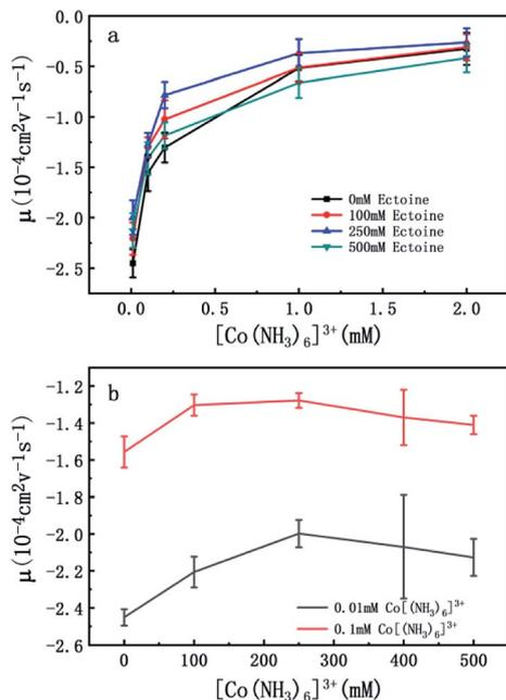
Fig. 4 (a) EM of DNA versus the concentration of  $[\text{Co}(\text{NH}_3)_6]^{3+}$  with 0 mM, 100 mM, 250 mM and 500 mM ectoine respectively. (b) EM of DNA versus the concentration of ectoine with 0.01 mM and 0.1 mM  $[\text{Co}(\text{NH}_3)_6]^{3+}$  respectively in solution. The error bars represent the corrected sample standard deviation.
