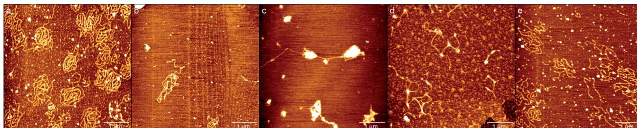
**Fig. 7** AFM images of DNA at different concentrations of ectoine and a fixed 0.01 mM [Co(NH<sub>3</sub>)<sub>6</sub>]<sup>3+</sup>. (a) Without ectoine. (b) 50 mM Ectoine. (c) 200 mM Ectoine. (d) 300 mM Ectoine. (e) 500 mM Ectoine. Buffer solution of Tris (10 mM, pH = 7.5) was used for all measurement.
