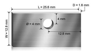
Fig. 1 Schematic showing the dimension of the machined Haynes 230 coupons used for corrosion where L is the length, W is the width, and D is the thickness of the coupons. A hole of 4 mm diameter is cut to allow the coupon to be hung on a Ni wire.
