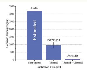
Fig. 4 Corrosion rates of Haynes 230 coupons in molten DC salts at  $800\pm10\,^{\circ}\text{C}$  for 100 hours following different purification treatments. Corrosion rate in non-treated DC salt was estimated at 3200  $\mu m$  per year or above.
