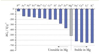
Fig. 5 Gibbs free energy of formation for different chlorides at 827  $^{\circ}$ C. The cations to the left of Mg<sup>2+</sup> are unstable in the presence of elemental Mg whereas the cations to the right of Mg<sup>2+</sup> are stable.
