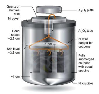
Fig. 2 Schematic of the corrosion vessel setup (not to scale) showing all components and spatial arrangement of Haynes 230 coupons and salts for corrosion tests. Mg chips are blended into the salt mixture.
