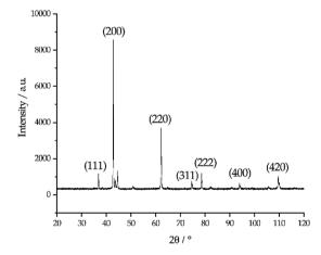
Fig. 7 X-ray diffraction pattern of the collected particles in the dark sludge phase. The numbers in the parentheses indicate the crystallographic orientations of MgO reference corresponding to each major diffraction peaks.
