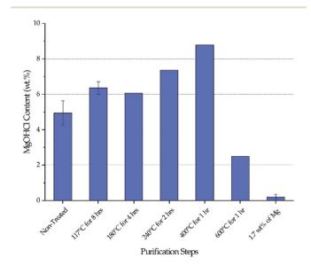
Fig. 3 Variation of MgOHCl during thermal purification and chemical purification with 1.7 wt% of Mg chips. The same batch of salt was used to obtain data at different purification steps. Error bars are present when multiple measurements were available.
