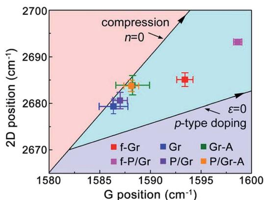
Fig. 4 A correlation map of the G and 2D peak positions of graphene at different steps in direct and PMMA-assisted transfer.
