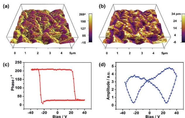
Fig. 2 PFM measurements of film **1**. (a) PFM phase mapping. (b) PFM amplitude mapping image overlaid on the 3D topography ( $5 \times 5 \mu\text{m}^2$ ). (c) PFM phase hysteresis loop. (d) PFM butterfly loop.
