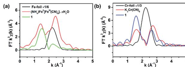
Fig. 3 Fourier transform (a) Fe K-edge and (b) Cr K-edge EXAFS of **1**,  $(\text{NH}_4)\text{Fe}[\text{Fe}(\text{CN})_4] \cdot x\text{H}_2\text{O}$ ,  $\text{K}_3\text{Cr}(\text{CN})_6$ , Fe foil and Cr foil respectively.
