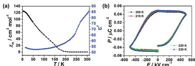
Fig. 5 (a) The temperature-dependent dielectric constant of the film 1 at  $f = 10$  kHz (blue), and thermal variation of  $\chi_m$  measured at 10 Oe (black), respectively. (b)  $P$ - $E$  hysteresis loop near the magnetic phase transition temperature of film 1.
