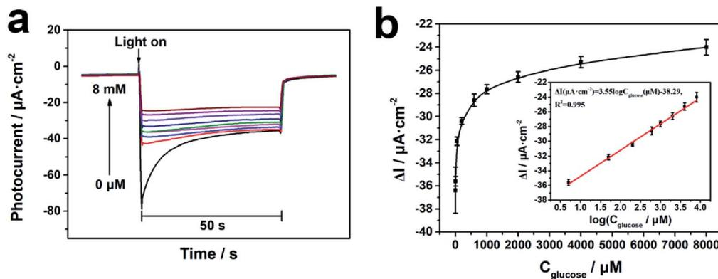
Fig. 4 PEC measurements of glucose by the PTEB photocathode. (a) The depressed photocurrent responses of the GOx modified PTEB photocathode at the applied bias of  $-0.3$  V with the increasing glucose concentration in air-saturated  $0.1$  M PBS (pH 7.0). (b) The corresponding plot of  $\Delta I$  vs. glucose concentration from  $5$   $\mu\text{M}$  to  $8$  mM and the calibration curve based on the calculation results (inset).
