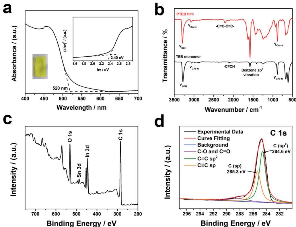
Fig. 2 Optical properties and chemical composition of PTEB photoelectrode. (a) UV-vis absorption spectrum of PTEB film covered on ITO electrode. Inset: the digital photograph and the  $(\alpha hv)^2$  vs.  $h\nu$  curve of PTEB film. (b) FT-IR spectra of TEB monomer (black) and PTEB film (red). XPS survey spectrum (c) and C 1s high-resolution XPS spectrum (d) of PTEB film on ITO substrate.
