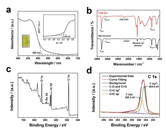
Fig. 2 Optical properties and chemical composition of PTEB photoelectrode. (a) UV-vis absorption spectrum of PTEB film covered on ITO electrode. Inset: the digital photograph and the  $(\alpha h v)^2$  vs. hv curve of PTEB film. (b) FT-IR spectra of TEB monomer (black) and PTEB film (red). XPS survey spectrum (c) and C 1s high-resolution XPS spectrum (d) of PTEB film on ITO substrate
