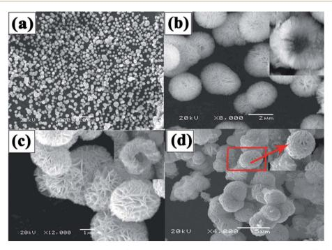
Fig. 3 (a) SEM image of the as-prepared precursor  $Ni(OH)_2$ . (b) Magnified SEM image of the as-prepared precursor  $Ni(OH)_2$ . (c) SEM image of NiO after being annealed at 400 °C. (d) SEM image of the  $NiO/MnO_2$  core-shell composite.
