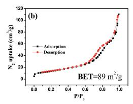
Fig. 2 Nitrogen adsorption—desorption isotherm of hollow NiO spheres (a). Nitrogen adsorption—desorption isotherm of the NiO/MnO $_2$  coreshell nanocomposite (b).
