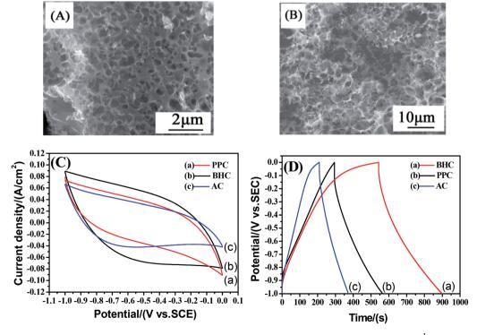
Fig. 7 SEM image of PPC (A). SEM image of BHC (B). CV curves of PPC, BHC and AC at the scan rates of 5 mV s $^{-1}$ , in 6.0 M KOH solution (C). Galvanostatic charge/discharge curves of PPC, BHC and AC at the current density of 5 mA cm $^{-2}$ , in 6.0 M KOH solution (D).
