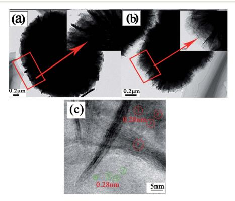
Fig. 4 (a) TEM image of NiO after being annealed at 400  $^{\circ}$ C. (b) TEM image of the NiO/MnO<sub>2</sub> core—shell composite. (c) HRTEM image of the NiO/MnO<sub>2</sub> core—shell composite.
