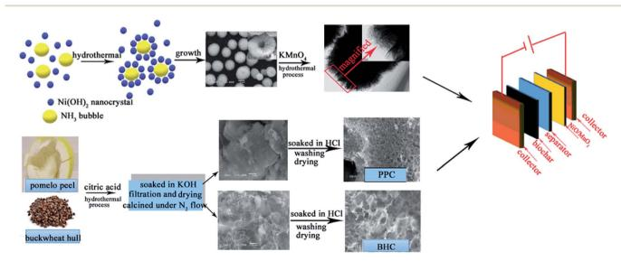
Scheme 1 Preparation process for the asymmetric supercapacitor device based on a core-shell NiO/MnO<sub>2</sub> cathode and biochar anode.
