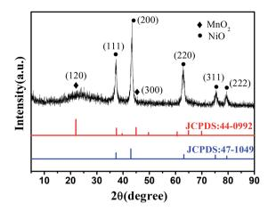
Fig. 1 XRD pattern of the NiO/MnO<sub>2</sub> core-shell nanocomposite.
