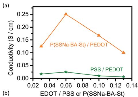
Fig. 3 (a) Conductivity of PSS/PEDOT and P(SSNa-BA-St)/PEDOT with the concentration ratio of EDOT increasing. (b) Relative weight ratio of three components and conductivities.
