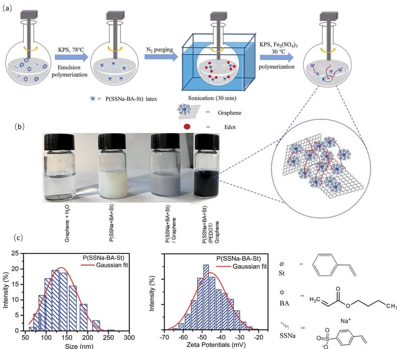
**Scheme 1** (a) Synthesis process of P(SSNa-BA-St)/PEDOT/graphene dispersions. (b) Photographs of dispersion of graphene in water, P(SSNa-BA-St) latex emulsions, P(SSNa-BA-St)/graphene and P(SSNa-BA-St)/PEDOT/graphene dispersions. (c) Hydrodynamic diameters and zeta potentials of P(SSNa-BA-St) latex.
