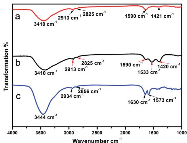
Fig. 4 FTIR spectra of the surface modified samples: NaYF<sub>4</sub>:Yb/Er@NaLuF<sub>4</sub>:Yb (a), UCNPs-OAO (b) and UCNPs-PEI (c).
