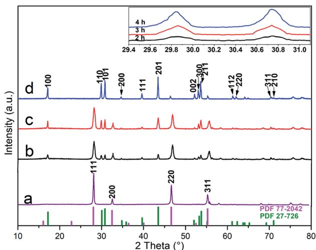
Fig. 1 XRD patterns of NaYF<sub>4</sub>:Yb/Er (a) and NaYF<sub>4</sub>:Yb/Er@NaLuF<sub>4</sub>:Yb with reaction time of 2 h (b), 3 h (c), 4 h (d), respectively. The inset shows a magnified patterns of  $2\theta$  about 30° and the bottom part is the lines pattern of the hexagonal phase (PDF 27-726) NaLuF<sub>4</sub> and cubic phase (PDF 77-2042) NaYF<sub>4</sub>, respectively.
