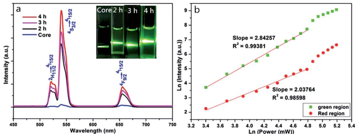
Fig. 3 Upconversion emission spectra of NaYF<sub>4</sub>:Yb/Er and NaYF<sub>4</sub>:Yb/Er@NaLuF<sub>4</sub>:Yb (0.3 g powder) with different reaction time excited by 980 nm CW diode laser (a); insets in (a) show luminescence photographs of UCNPs dispersed in cyclohexane. Red and green emission intensity relationship with dependence of the laser pump power for the NaYF<sub>4</sub>:Yb/Er@NaLuF<sub>4</sub>:Yb with reaction time of 4 h (b).
