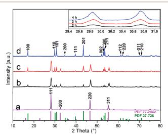
Fig. 1 XRD patterns of NaYF<sub>4</sub>:Yb/Er (a) and NaYF<sub>4</sub>:Yb/Er@NaLuF<sub>4</sub>:Yb with reaction time of 2 h (b), 3 h (c), 4 h (d), respectively. The inset shows a magnified patterns of  $2\theta$  about  $30^{\circ}$ C and the bottom part is the lines pattern of the hexagonal phase (PDF 27-726) NaLuF<sub>4</sub> and cubic phase (PDF 77-2042) NaYF<sub>4</sub>, respectively.
