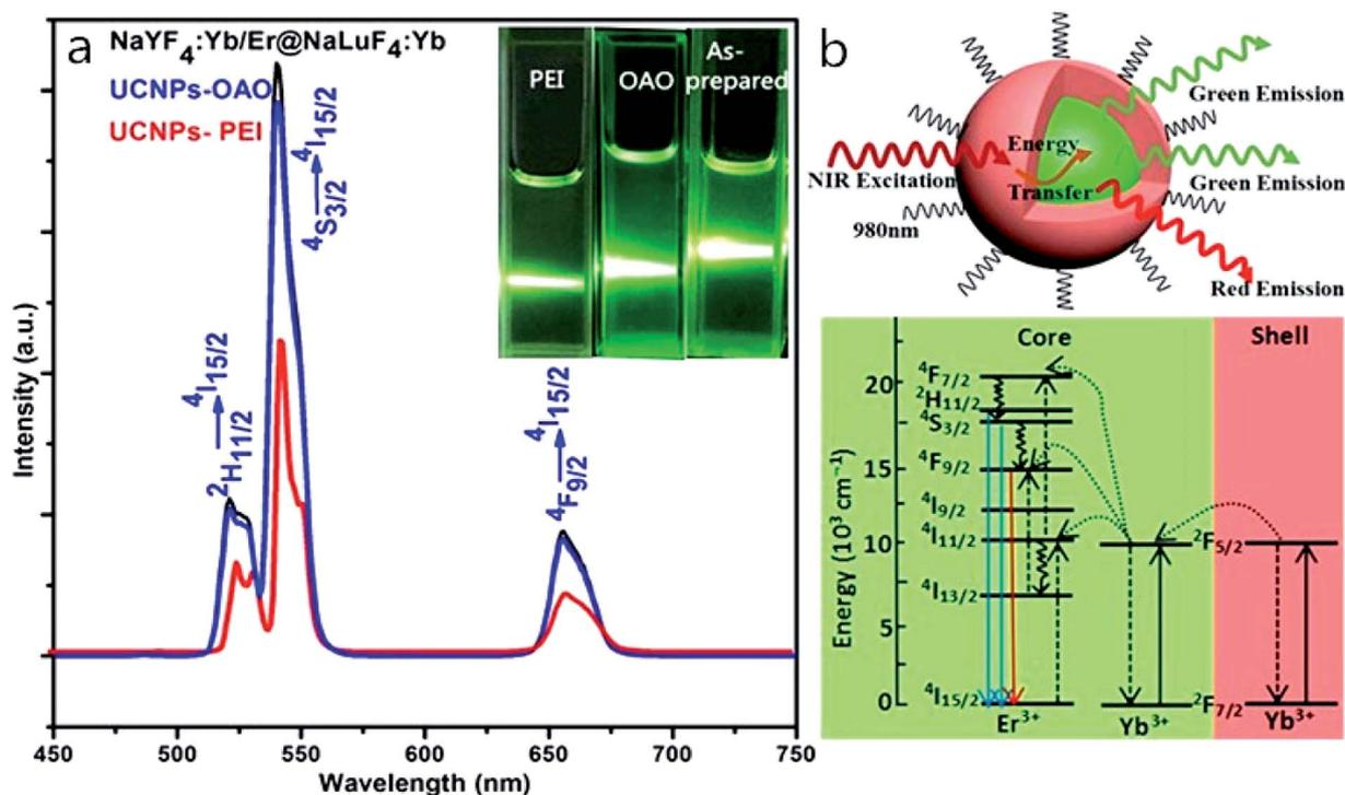
Fig. 5 Upconversion emission spectra of  $\text{NaYF}_4:\text{Yb}/\text{Er}@\text{NaLuF}_4:\text{Yb}$ , UCNPs-PEI and UCNPs-OAO (0.3 g powder) excited by 980 nm CW diode laser (a). Insets in (a) show luminescence photographs of UCNPs dispersed in cyclohexane or water. Schematic illustration and energy level diagram (bottom) of core-shell nanoparticles excited by 980 nm laser (b).
