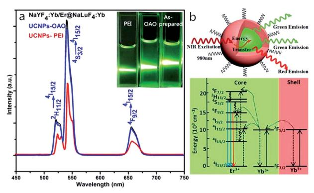
Fig. 5 Upconversion emission spectra of NaYF<sub>4</sub>:Yb/Er@NaLuF<sub>4</sub>:Yb, UCNPs-PEI and UCNPs-OAO (0.3 g powder) excited by 980 nm CW diode laser (a). Insets in (a) show luminescence photographs of UCNPs dispersed in cyclohexane or water. Schematic illustration and energy level diagram (bottom) of core-shell nanoparticles excited by 980 nm laser (b).
