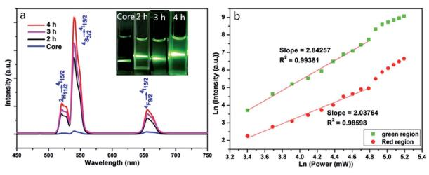
Fig. 3 Upconversion emission spectra of NaYF<sub>4</sub>:Yb/Er and NaYF<sub>4</sub>:Yb/Er@NaLuF<sub>4</sub>:Yb (0.3 g powder) with different reaction time excited by 980 nm CW diode laser (a); insets in (a) show luminescence photographs of UCNPs dispersed in cyclohexane. Red and green emission intensity relationship with dependence of the laser pump power for the NaYF<sub>4</sub>:Yb/Er@NaLuF<sub>4</sub>:Yb with reaction time of 4 h (b).
