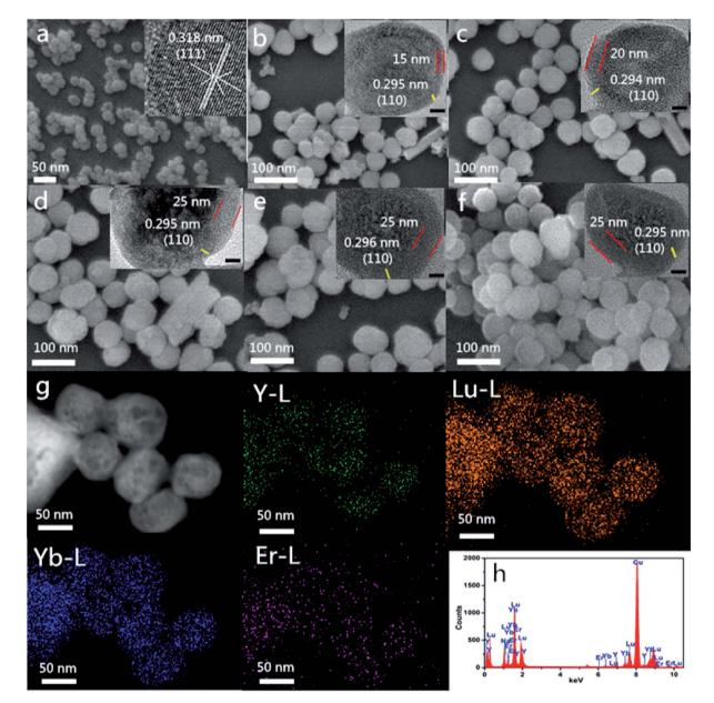
Fig. 2 SEM images of NaYF<sub>4</sub>:Yb/Er (a), NaYF<sub>4</sub>:Yb/Er@NaLuF<sub>4</sub>:Yb with reaction time of 2 h (b), 3 h (c), 4 h (d), UCNPs-OAO (e), UCNPs-PEI (f), respectively; elemental mapping and EDS of NaYF<sub>4</sub>:Yb/Er@NaLuF<sub>4</sub>:Yb with reaction time of 4 h (g) and (h), respectively. Insets in (a)–(f) show HR-TEM images of UCNPs. Scale bars represent 20 nm for insets.
