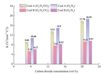
Fig. 6 Relationship between the comprehensive combustion performance index and  ${\rm O}_2$  concentration.
