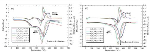
Fig. 3 DSC and DDSC curves of the two coal samples with the heating rate of 5 °C min<sup>-1</sup> under different atmospheres, (a) coal A and (b) coal B.
