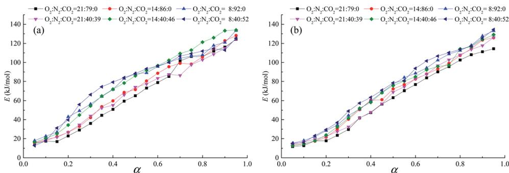
Fig. 8 Relationship between apparent activation energy and conversion during the oxygen-adsorption stage (stage 2), (a) coal A and (b) coal B.
