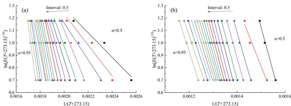
Fig. 7 Linear relationship between  $\ln(\beta/(T + 273.15)^{1.92})$  and  $1/(T + 273.15)$  of coal A in atmosphere O<sub>2</sub> : N<sub>2</sub> : CO<sub>2</sub> = 21 : 40 : 39, (a) in oxygen-adsorption stage and (b) combustion domain stage.
