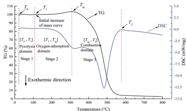
Fig. 1 TG and DSC curves of a coal sample showing the temperature boundaries for different stages. This individual diagram is obtained from the thermal analysis of coal A conversion under 21 vol% O<sub>2</sub>/79 vol% N<sub>2</sub> and heating rate of 5 °C min<sup>-1</sup>.
