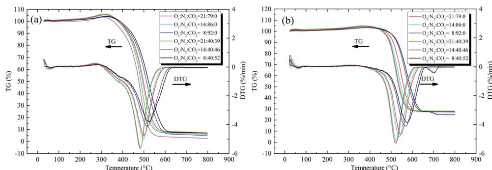
Fig. 2 TG and DTG curves of the two coal samples with the heating rate of 5 °C min<sup>-1</sup> under different atmospheres, (a) coal A and (b) coal B.
