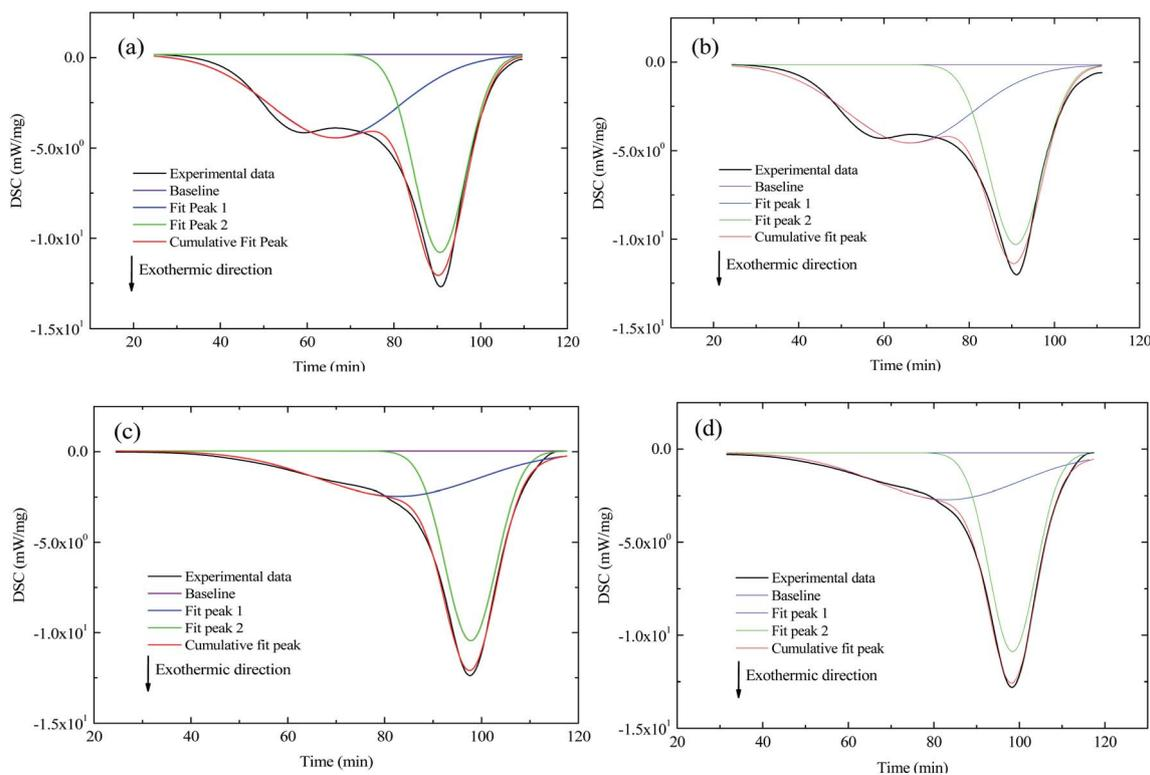
Fig. 4 DSC curves from the pyrolysis domain stage (stage 1) through the combustion domain stage (stage 3) for the two coal samples, (a) coal A in atmosphere  $\text{O}_2 : \text{N}_2 = 21 : 79$ , (b) coal A in atmosphere  $\text{O}_2 : \text{N}_2 : \text{CO}_2 = 21 : 40 : 39$ , (c) coal B in atmosphere  $\text{O}_2 : \text{N}_2 = 21 : 79$ , and (d) coal B in atmosphere  $\text{O}_2 : \text{N}_2 : \text{CO}_2 = 21 : 40 : 39$ .
