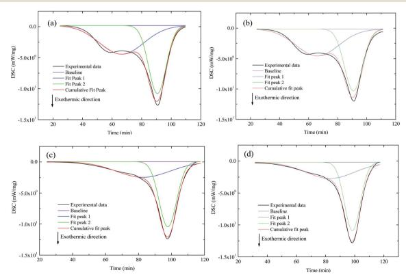
Fig. 4 DSC curves from the pyrolysis domain stage (stage 1) through the combustion domain stage (stage 3) for the two coal samples, (a) coal A in atmosphere  $O_2: N_2 = 21:79$ , (b) coal A in atmosphere  $O_2: N_2 = 21:40:39$ , (c) coal B in atmosphere  $O_2: N_2 = 21:79$ , and (d) coal B in atmosphere  $O_2: N_2: CO_2 = 21:40:39$ .
