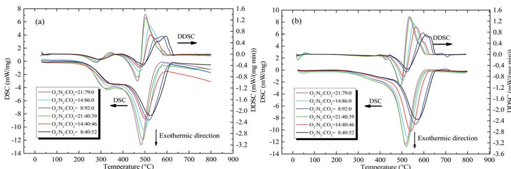
Fig. 3 DSC and DDSC curves of the two coal samples with the heating rate of 5 °C min<sup>-1</sup> under different atmospheres, (a) coal A and (b) coal B.
