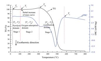
Fig. 1 TG and DSC curves of a coal sample showing the temperature boundaries for different stages. This individual diagram is obtained from the thermal analysis of coal A conversion under 21 vol%  $O_2/79$  vol%  $N_2$  and heating rate of 5 °C min<sup>-1</sup>.
