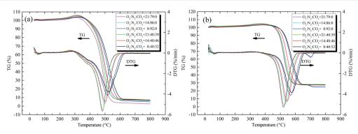
Fig. 2 TG and DTG curves of the two coal samples with the heating rate of 5 °C min<sup>-1</sup> under different atmospheres, (a) coal A and (b) coal B.
