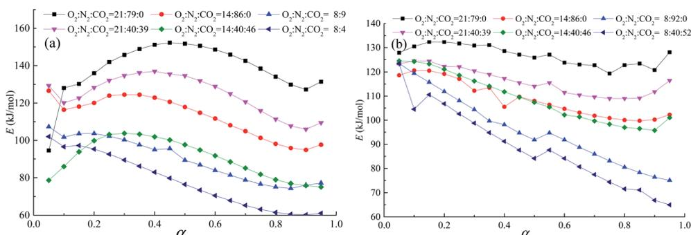
Fig. 9 Relationship between apparent activation energy and conversion during the combustion domain stage (stage 3), (a) coal A and (b) coal B.
