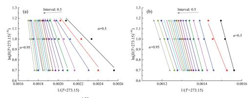
Fig. 7 Linear relationship between  $\ln(\beta/(T+273.15)^{1.92})$  and 1/(T+273.15) of coal A in atmosphere  $O_2: N_2: CO_2=21: 40: 39$ , (a) in oxygen-adsorption stage and (b) combustion domain stage.
