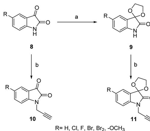
Scheme 2 Syntheses of *N*-propargylated C-5-substituted isatin **10** and spiroketal-*N*-propargylated C-5-substituted isatin **11**. Reagents and conditions: (a) 2-bromoethan-1-ol, NaH, DMF, 80 °C, 6 h. (b) Propargyl bromide, NaH, DMF, 80 °C, 6 h.
