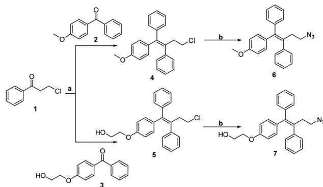
Scheme 1 Synthesis of ospemifene and the *O*-methoxy derivative of ospemifene. Reagents and conditions: (a) Zn/TiCl<sub>4</sub>, anhydrous THF, rt to reflux, 6 h. (b) NaN<sub>3</sub>, DMF, 60 °C, 4 h.
