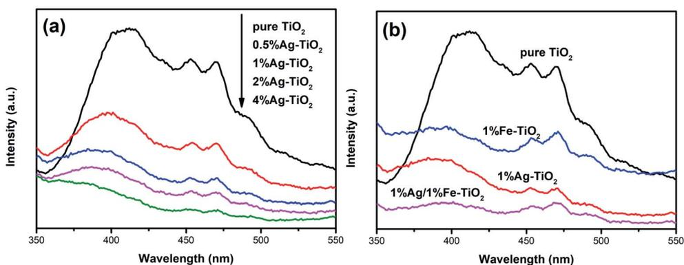
Fig. 8 PL spectra of (a) Ag-TiO<sub>2</sub>, (b) pure TiO<sub>2</sub>, 1% Ag-TiO<sub>2</sub>, 1% Fe-TiO<sub>2</sub> and 1% Ag/1% Fe-TiO<sub>2</sub>.
