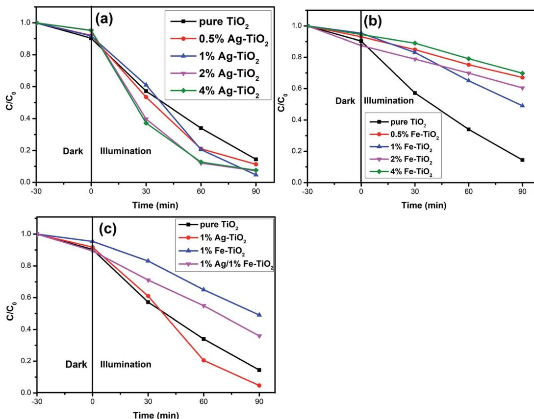
Fig. 6 Decolorization rate curves of RhB for (a) Ag-TiO<sub>2</sub>, (b) Fe-TiO<sub>2</sub>, and (c) 1% Ag/1% Fe-TiO<sub>2</sub>.
