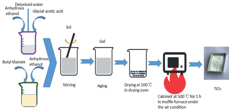
Fig. 1 The preparation process of TiO<sub>2</sub>.
