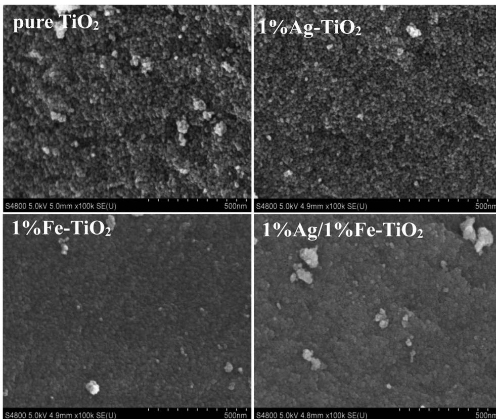
Fig. 4 SEM images of pure TiO<sub>2</sub>, 1% Ag–TiO<sub>2</sub>, 1% Fe–TiO<sub>2</sub> and 1% Ag/1% Fe–TiO<sub>2</sub>.
