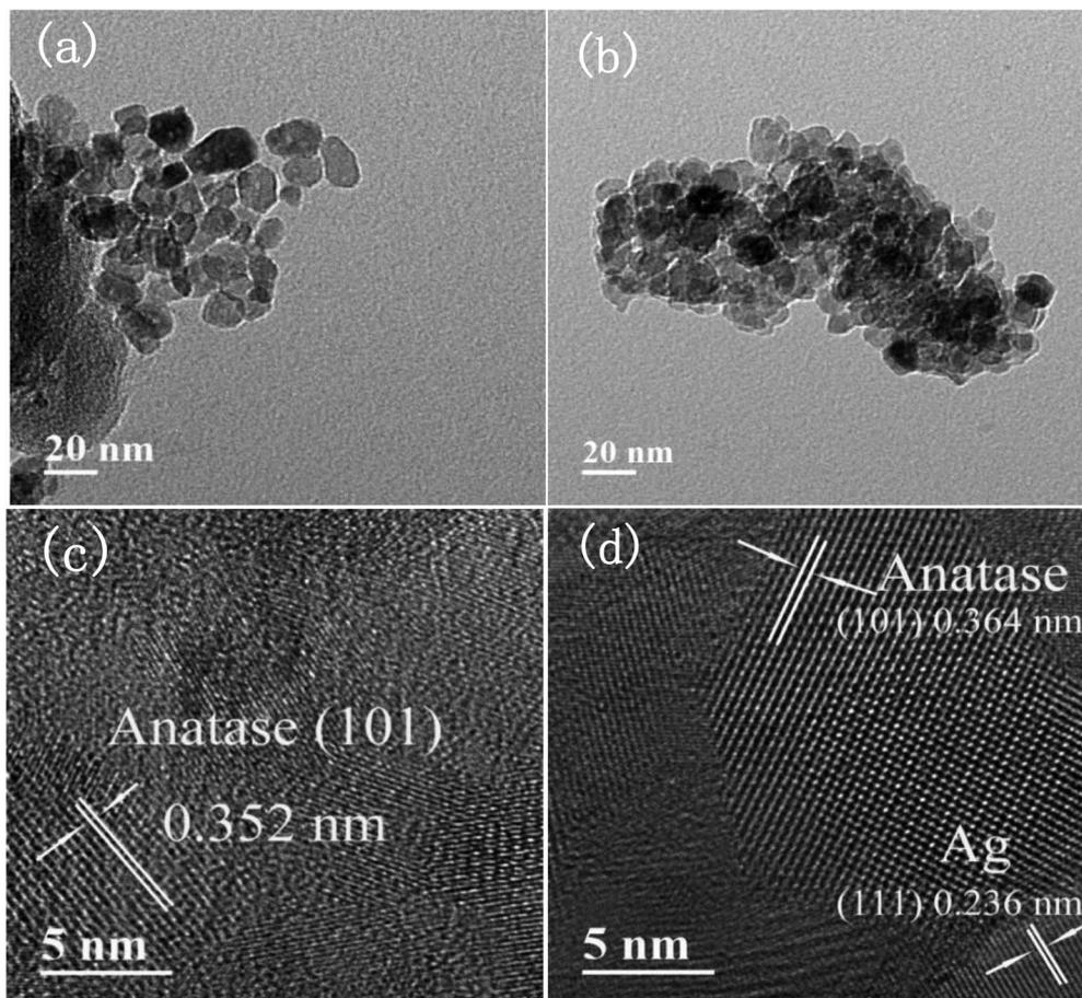
Fig. 5 TEM images of (a) pure TiO<sub>2</sub>, (b) 1% Ag/1% Fe-TiO<sub>2</sub>, HRTEM images of (c) pure TiO<sub>2</sub>, and (d) 1% Ag/1% Fe-TiO<sub>2</sub>.
