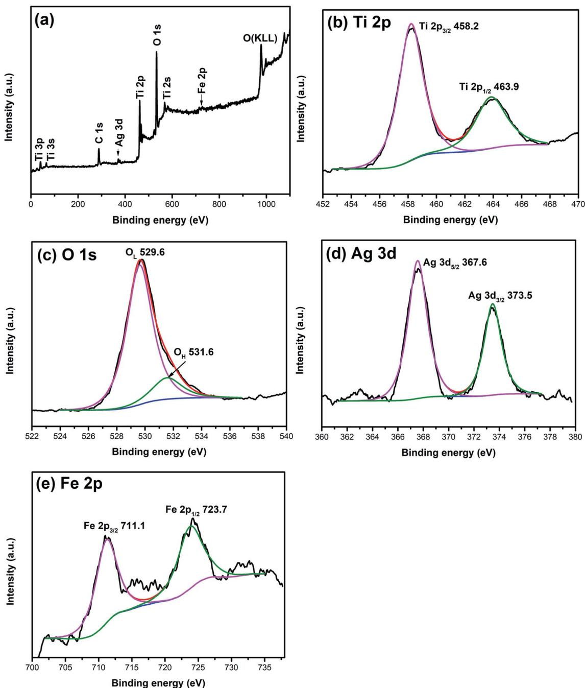
Fig. 3 XPS spectra of 1% Ag/1% Fe-TiO<sub>2</sub>: (a) total spectrum, (b) Ti 2p, (c) O 1s, (d) Ag 3d and (e) Fe 2p.
