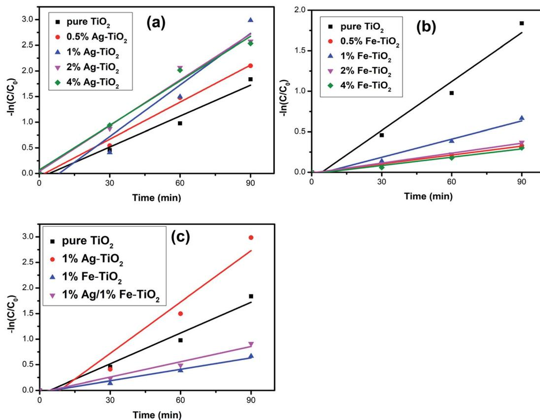
Fig. 7 Kinetics linear simulation curves of (a) Ag-TiO<sub>2</sub>, (b) Fe-TiO<sub>2</sub>, and (c) 1% Ag/1% Fe-TiO<sub>2</sub>.
