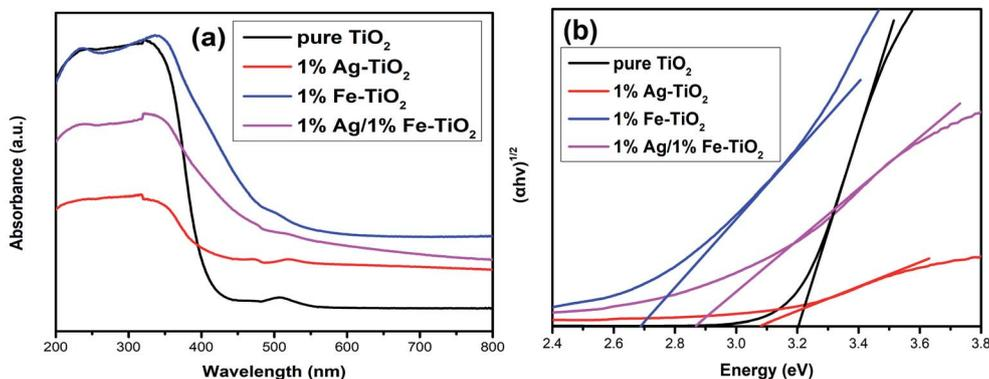
Fig. 9 (a) UV-visible absorption spectra and (b) plots of  $(\alpha h\nu)^{1/2}$  versus energy ( $h\nu$ ) of pure TiO<sub>2</sub>, 1% Ag-TiO<sub>2</sub>, 1% Fe-TiO<sub>2</sub> and 1% Ag/1% Fe-TiO<sub>2</sub>.
