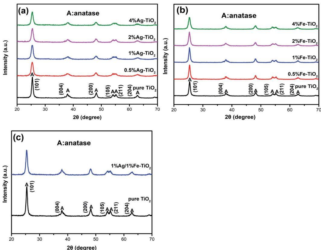
Fig. 2 XRD patterns of (a) Ag-TiO<sub>2</sub>, (b) Fe-TiO<sub>2</sub> and (c) 1% Ag/1% Fe-TiO<sub>2</sub>.
