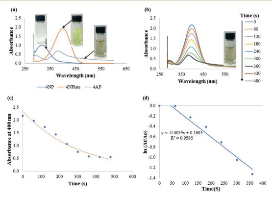
Fig. 5 (a) UV-vis absorption plot of 4 NP, 4 NPlate and 4 AP. Inset shows the photographic images (b) UV-vis absorption spectra of 4 NPlate reduction with time. Inset shows the photographic image of the degradation product (c) plot of absorbance at 400 nm with time and (d) linear plot of  $ln(A_t/A_o)$  vs. time.
