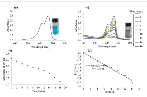
Fig. 6 (a) UV-vis absorption plot of MB. Inset shows the photographic image (b) UV-vis absorption spectra of MB reduction with time. Inset shows the photographic image of the degradation product (c) plot of absorbance at 664 nm with time and (d) linear plot of  $\ln(A_1/A_0)$  vs. time.
