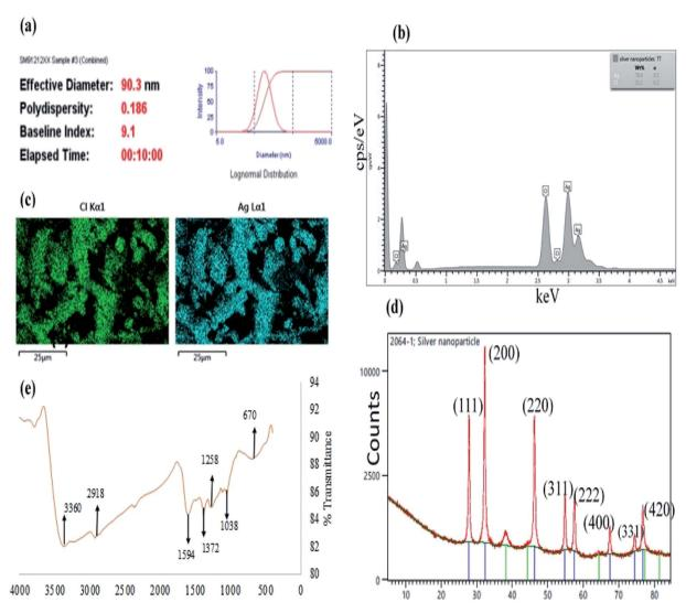
Fig. 4 (a) Particles diameter estimate of CAPE-AgNPs from DLS (b) energy dispersive X-ray analysis of CAPE-AgNPs (c) selected elemental mapping of CAPE-AgNPs (d) FTIR Spectrum of CAPE-AgNPs and (e) X-ray diffraction of CAPE-AgNPs.
