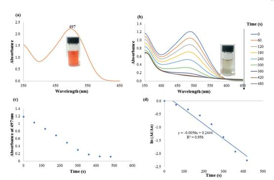
Fig. 7 (a) UV-vis absorption plot of CR. Inset shows the photographic image (b) UV-vis absorption spectra of CR reduction with time. Inset shows the photographic image of the degradation product (c) plot of absorbance at 497 nm with time and (d) linear plot of  $\ln(A_t/A_0)$  vs. time.
