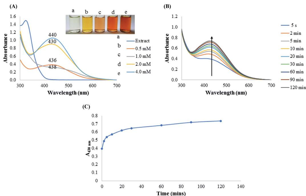
Fig. 2 (A) Synthesis of CAPE-AgNPs under different concentrations of  $\text{AgNO}_3$ . Inset shows the photographic images of CAPE-AgNPs with (a) CAPE extract (b) 0.5 mM (c) 1.0 mM (d) 2.0 mM and (e) 4.0 mM  $\text{AgNO}_3$  (B) kinetics of CAPE-AgNPs synthesis under 2.0 mM  $\text{AgNO}_3$  within time of 0–120 min and (C) Plot of absorbance at 400 nm of CAPE-AgNPs with time.
