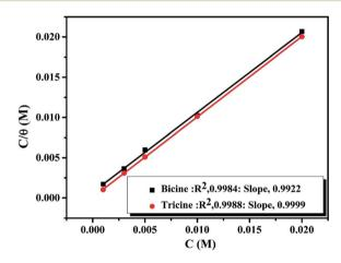
Fig. 7 Langmuir isotherms for the adsorption of bicine and tricine on the copper surface in stagnant naturally aerated neutral 3.5 mass% NaCl solutions at 25  $^{\circ}$ C.
