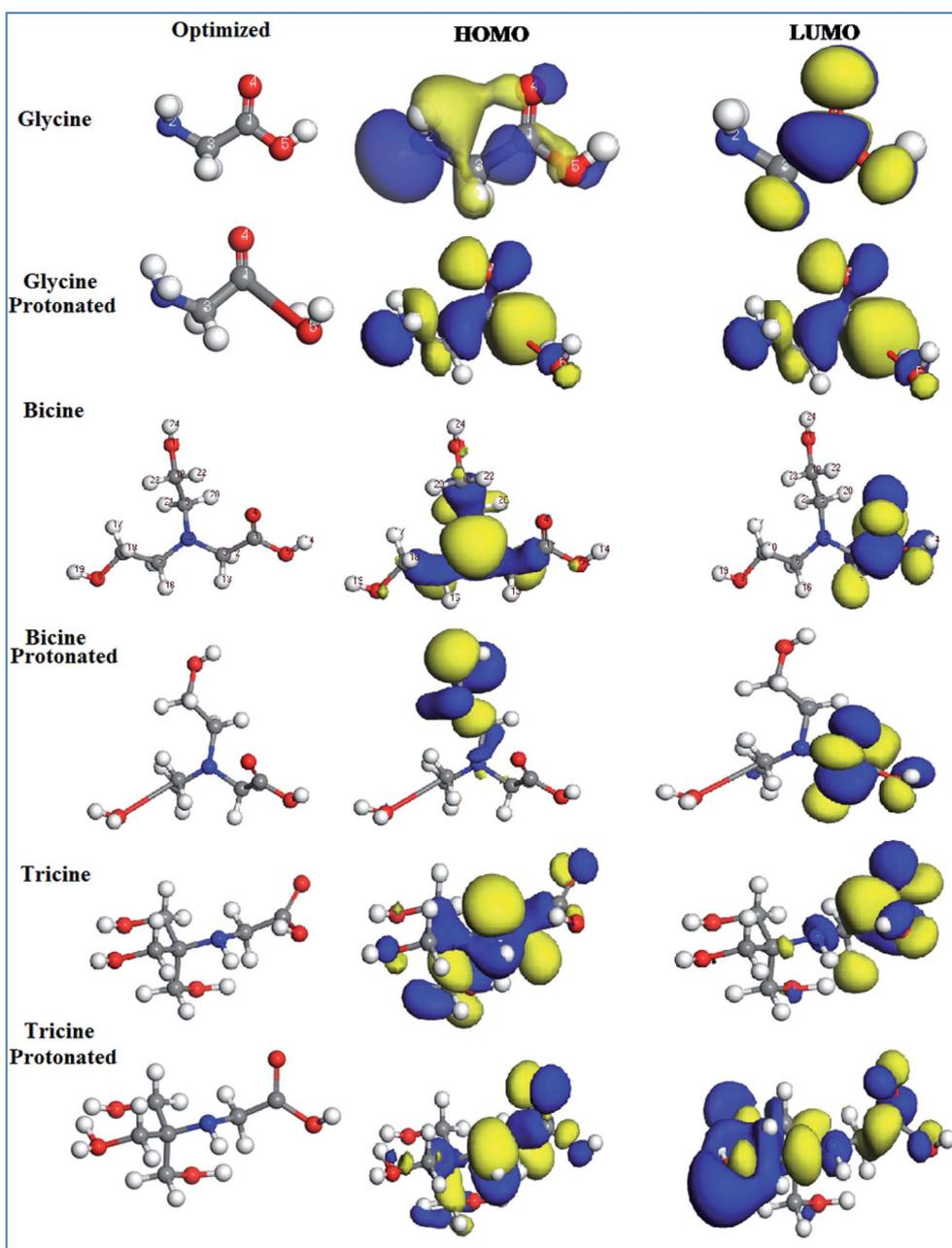
Fig. 8 The optimized structures and the frontier molecular orbitals (HOMO and LUMO) for the gas, solvated and protonated species obtained with DFT/GGA/DNP 4.4.
