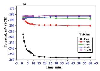
Fig. 2 Variation of the open circuit potential of a copper electrode in stagnant naturally aerated 3.5 mass% NaCl solutions in the absence and presence of different concentrations of bicine (a) and tricine (b).
