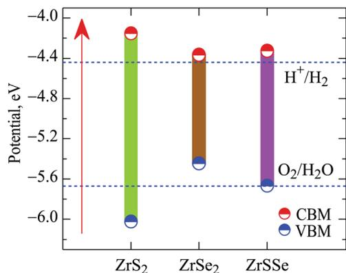
Fig. 5 The VBM and CBM edge alignment of  $\text{ZrS}_2$ ,  $\text{ZrSe}_2$ , and Janus  $\text{ZrSSe}$  monolayers. The horizontal dashed lines refer to the standard potentials for water splitting at pH = 0.
