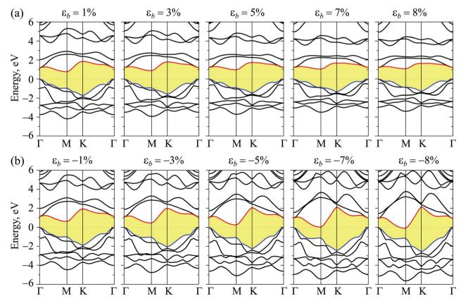
Fig. 6 Band structure of the Janus ZrSSe under different levels of (a) tensile, and (b) compressive biaxial strains.
