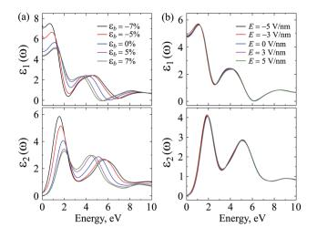
Fig. 10 Dielectric function parts of Janus ZrSSe under (a) biaxial strain, and (b) electric field.
