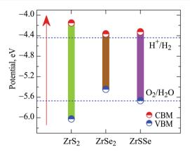
Fig. 5 The VBM and CBM edge alignment of  $ZrS_2$ ,  $ZrSe_2$ , and Janus ZrSSe monolayers. The horizontal dashed lines refer to the standard potentials for water splitting at pH = 0.
