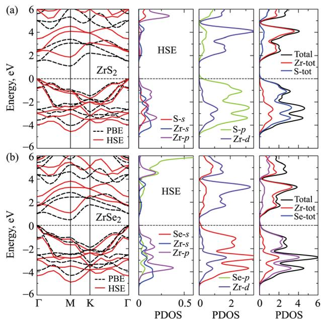
**Fig. 3** Band structures and PDOS of the monolayers ZrS<sub>2</sub> (a), and ZrSe<sub>2</sub> (b). The Fermi level is set to be zero.
