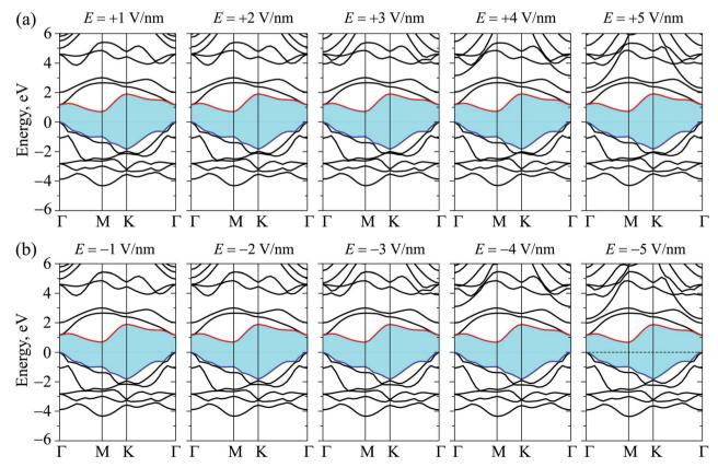
Band structure of the Janus ZrSSe under (a) positive, and (b) negative, external electric fields.
