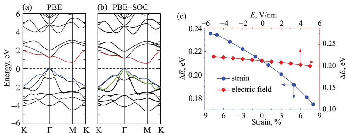
Fig. 9 Calculated band structures of the Janus ZrSSe using (a) PBE, and (b) PBE + SOC methods. Effect of biaxial strain and electric field on the spin–orbit splitting value  $\Delta E$  at the  $\Gamma$ -point using PBE + SOC of the Janus ZrSSe (c).
