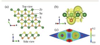
Fig. 1 (a) Optimized atomic structure of Janus ZrSSe, (b) charge density in the Janus ZrSSe with isolated 0.04, and (c) electron density of atoms in contour form from 0 to 0.2 e  $Bohr^{-3}$  with the interval of 0.02  $Bohr^3$ .
