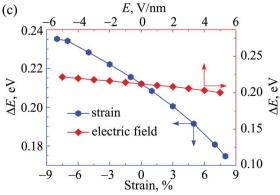
Fig. 9 Calculated band structures of the Janus ZrSSe using (a) PBE, and (b) PBE + SOC methods. Effect of biaxial strain and electric field on the spin-orbit splitting value  $\Delta E$  at the  $\Gamma$ -point using PBE + SOC of the Janus ZrSSe (c).
