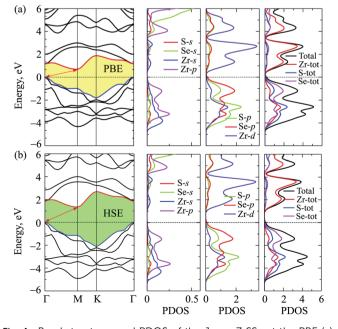
Fig. 4 Band structures and PDOS of the Janus ZrSSe at the PBE (a), and HSE (b) levels.
