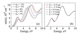
Fig. 11 Absorption coefficient  $\alpha(\omega)$  of Janus ZrSSe under (a) biaxial stain, and (b) electric field.
