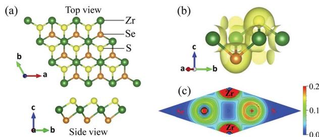
Fig. 1 (a) Optimized atomic structure of Janus ZrSSe, (b) charge density in the Janus ZrSSe with isolated  $0.04$ , and (c) electron density of atoms in contour form from  $0$  to  $0.2 \text{ e Bohr}^{-3}$  with the interval of  $0.02 \text{ Bohr}^{-3}$ .
