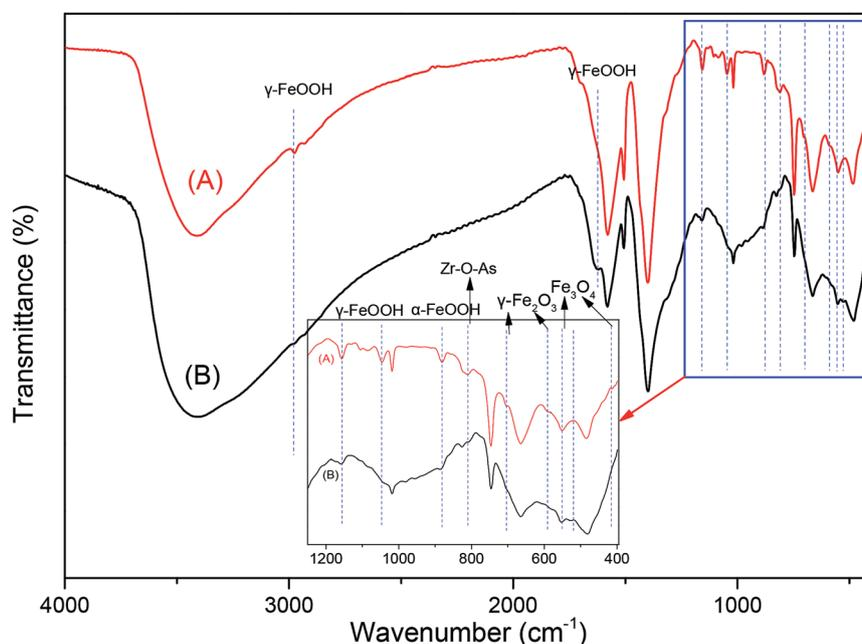
Fig. 6 FTIR of fresh MOFs-NZVI (A) and MOFs-NZVI (B) reacted with As(III) after 60 min. Inset: the spectra from 395–1200  $\text{cm}^{-1}$  is enlarged ( $m_{\text{MOFs-NZVI}} = 0.15$  g, mass fraction of NZVI = 16.7%,  $C_{\text{As(III)}} = 20$  mg  $\text{L}^{-1}$ ,  $V_{\text{As(III)}} = 100$  mL, pH = 7.0,  $T = 25$  °C).
