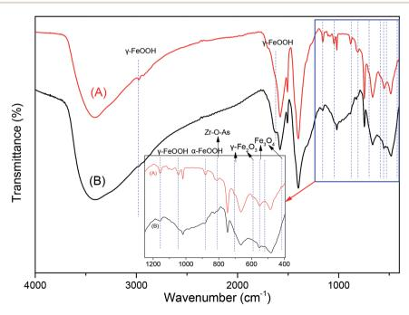
Fig. 6 FTIR of fresh MOFs-NZVI (A) and MOFs-NZVI (B) reacted with As(III) after 60 min. Inset: the spectra from  $395-1200 \, \text{cm}^{-1}$  is enlarged ( $m_{\text{MOFs}-1}$ ) after 60 min. Inset: the spectra from  $395-1200 \, \text{cm}^{-1}$ ) is enlarged ( $m_{\text{MOFs}-1}$ ).  $_{NZVI} = 0.15$  g, mass fraction of NZVI = 16.7%,  $C_{As(III)} = 20$  mg L<sup>-1</sup>,  $V_{As(III)} = 100$  mL, pH = 7.0, T = 25 °C).
