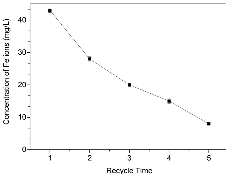
Fig. 10 The concentration of Fe ions in the leaching solution after each recycle ( $m_{\text{MOFs-NZVI}} = 0.15$  g, mass fraction of NZVI = 16.7%,  $C_{\text{As(III)}} = 20$  mg  $\text{L}^{-1}$ ,  $V_{\text{As(III)}} = 100$  mL, pH = 7.0,  $T = 25$  °C,  $t = 60$  min).
