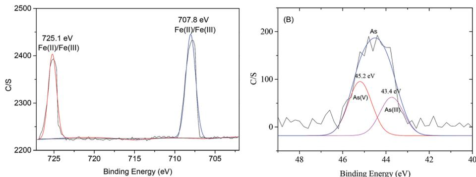
Fig. 7 High-resolution XPS survey of (A) Fe 2p<sub>3</sub> and (B) As 3d for MOFs-NZVI reaction with As(III) after 60 min ( $m_{\text{MOFs-NZVI}} = 0.15$  g, mass fraction of NZVI = 16.7%,  $C_{\text{As(III)}} = 20$  mg L<sup>-1</sup>,  $V_{\text{As(III)}} = 100$  mL, pH = 7.0,  $T = 25$  °C).
