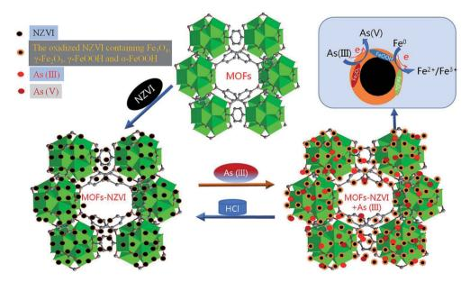
Fig. 8 Schematic diagram showing the removal mechanism of As(III) using MOFs-NZVI.
