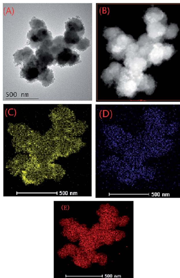
Fig. 3 (A) TEM image and (B) HADDF image of MOFs-NZVI reacted with As(III), elemental mappings of (C) Fe, (D) As and (E) Zr ( $m_{MOFs-NZVI} = 0.15$  g, mass fraction of NZVI = 16.7%,  $C_{As(III)} = 20$  mg L<sup>-1</sup>,  $V_{As(III)} = 100$  mL, pH = 7.0,  $T = 25$  °C).
