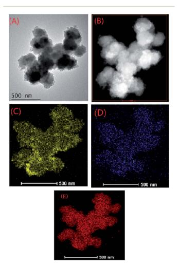
Fig. 3 (A) TEM image and (B) HADDF image of MOFs-NZVI reacted with As(III), elemental mappings of (C) Fe, (D) As and (E) Zr ( $m_{\text{MOFs-NZVI}} = 0.15$  g, mass fraction of NZVI = 16.7%,  $C_{\text{As(III)}} = 20$  mg L $^{-1}$ ,  $V_{\text{As(III)}} = 100$  mL, pH = 7.0, T = 25 °C).
