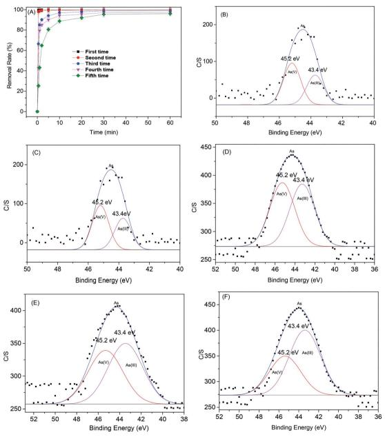
Fig. 9 (A) As(III) removal efficiency in each cycle after regeneration using MOFs-NZVI, high-resolution XPS survey of As 3d for MOFs-NZVI reaction with As(III) after 60 min at the first time (B), the second time (C), the third time (D), the fourth time (E) and the fifth time (F) (m<sub>MOFs-NZVI</sub> = 0.15 g, mass fraction of NZVI = 16.7%,  $C_{As(III)} = 20$  mg L<sup>-1</sup>,  $V_{As(III)} = 100$  mL, pH = 7.0, T = 25 °C).
