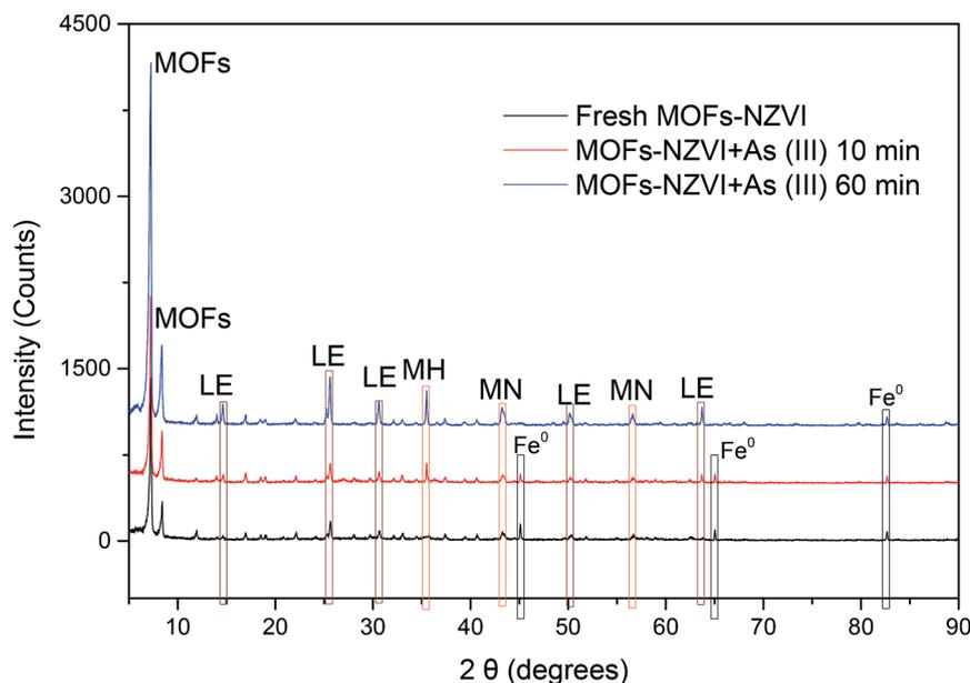
Fig. 5 X-ray diffraction patterns of fresh MOFs-NZVI, MOFs-NZVI reacted with As(III) after 10 min and 60 min. Peaks are due to NZVI ( $\text{Fe}^0$ ), magnetite ( $\text{Fe}_3\text{O}_4$ ) (MN), maghemite ( $\gamma\text{-Fe}_2\text{O}_3$ ) (MH), lepidocrocite ( $\gamma\text{-FeOOH}$ ) (LE), respectively ( $m_{\text{MOFs-NZVI}} = 0.15$  g, mass fraction of NZVI = 16.7%,  $C_{\text{As(III)}} = 20$  mg  $\text{L}^{-1}$ ,  $V_{\text{As(III)}} = 100$  mL, pH = 7.0,  $T = 25$  °C).
