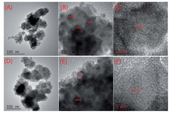
Fig. 2 TEM images of (A)–(C) of fresh MOFs-NZVI and (D)–(F) of MOFs-NZVI reacted with As(III) ( $m_{\text{MOFs-NZVI}} = 0.15$  g, mass fraction of NZVI = 16.7%,  $C_{\text{As(III)}} = 20$  mg L<sup>-1</sup>,  $V_{\text{As(III)}} = 100$  mL, pH = 7.0, T = 25 °C).
