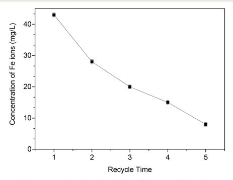
Fig. 10 The concentration of Fe ions in the leaching solution after each recycle  $(m_{MOFs-NZVI} = 0.15 \text{ g}, \text{ mass fraction of NZVI} = 16.7\%, C_{As(m)} = 1.00 \text{ mass fraction of NZVI}$ 20 mg L<sup>-1</sup>,  $V_{As(III)} = 100$  mL, pH = 7.0, T = 25 °C, t = 60 min).
