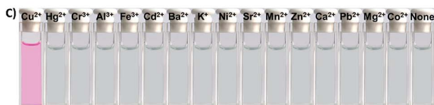
Fig. 5 (A) Absorption spectra of 1o (20 \mu\text{M} ) in the presence of various metal ions (10.0 equiv.) in THF. (B) Effect of competitive metal ions on the interaction between 1o and \text{Cu}^{2+} ion. (C) The color of 1o upon addition of various metal ions.
