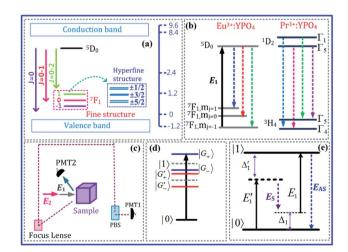
Fig. 1 (a) Fine and hyperfine energy level of  $Eu^{3+}$ :YPO<sub>4</sub>. (b) Energy level diagram of  $Eu^{3+}$ :YPO<sub>4</sub> and  $Pr^{3+}$ :YPO<sub>4</sub>. <sup>22-24</sup> (c) Schematic diagram of experimental setup. (d) Four-wave mixing (FWM) of lambda level system. (e) FWM in a two-level system.
