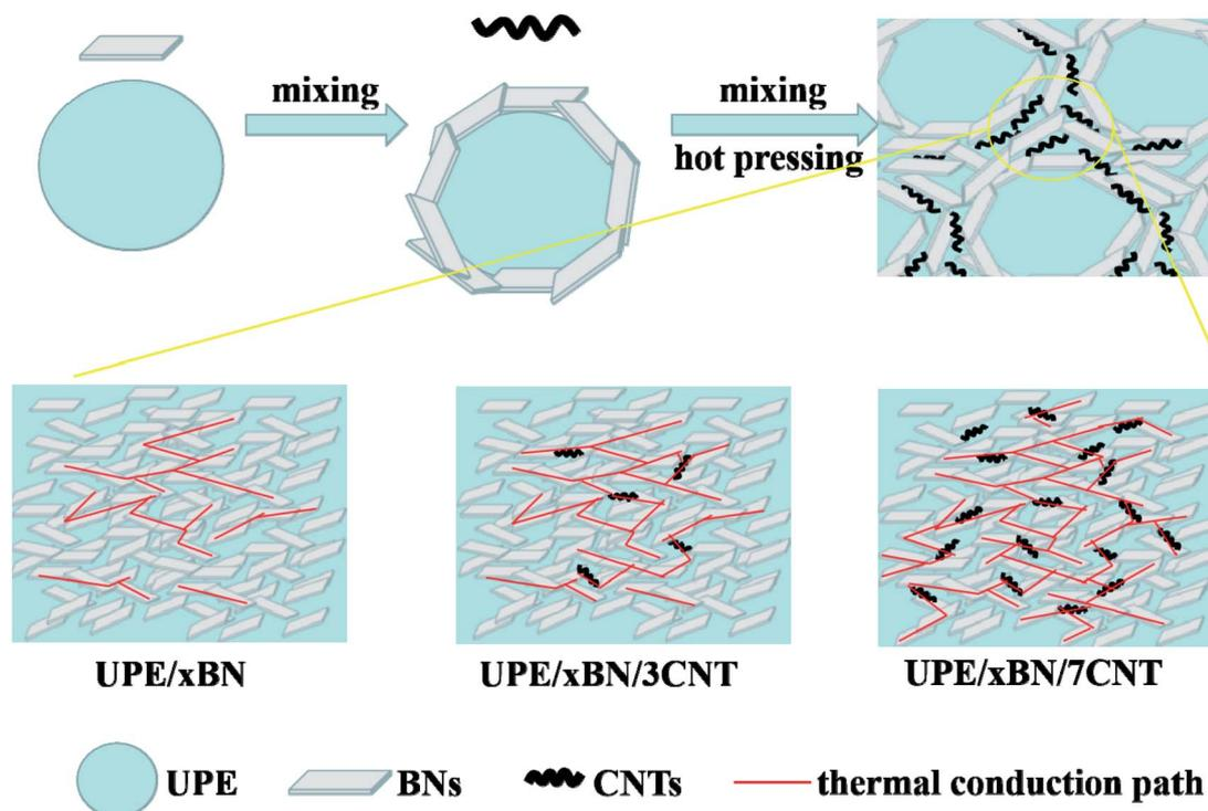
**Fig. 8** Schematic diagram of preparation process and heat transport pathways of UPE/BN/CNT composites.
