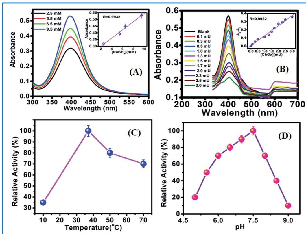
Fig. 8 UV-visible spectra of (A)  $\text{AgNO}_3$  with various concentrations of  $\text{NaBH}_4$  and (B) AgNPs with various concentrations of ChOx in the presence of cholesterol. Relative enzymatic activity of ChOx as a function of (C) temperature and (D) pH.
