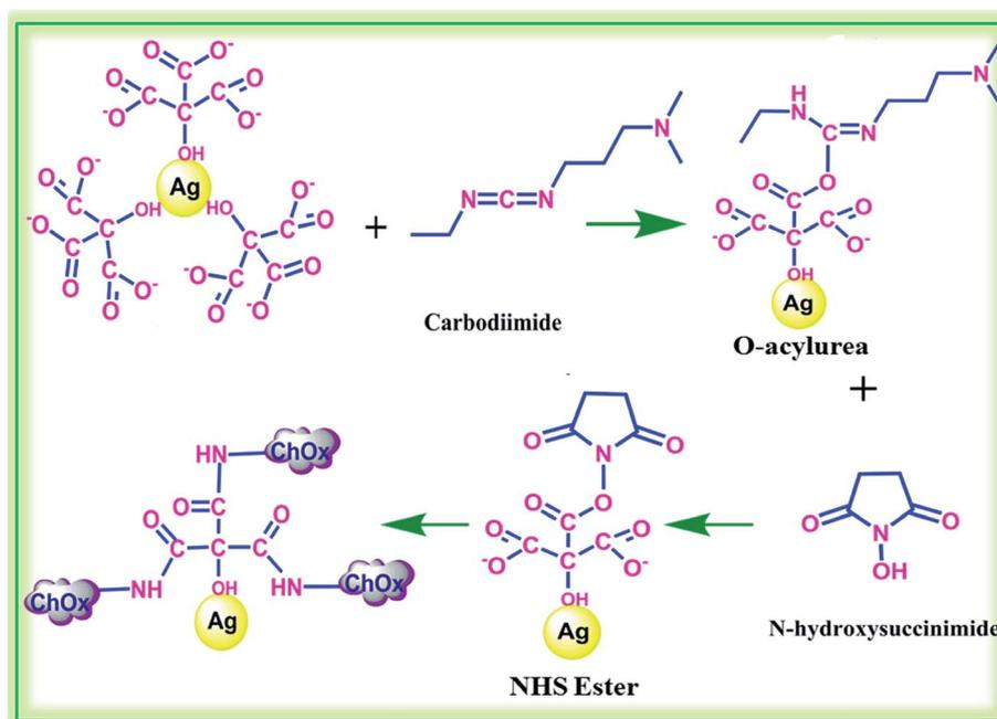
Fig. 3 Activation of functional groups on the surfaces of AgNPs using EDC/NHS and conjugation with ChOx.
