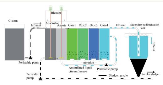
Fig. 1 Schematic diagram of the A/A/O system.
