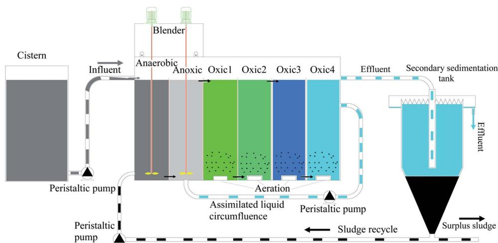
Fig. 1 Schematic diagram of the A/A/O system.
