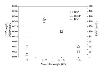
Fig. 4 Distribution of DBP and DEHP in different MW fractions of DOC in raw leachate.
