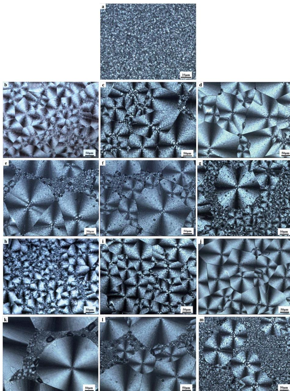
Fig. 4 POM photomicrograph of PCL undergone a program cooling ( $10^\circ\text{C min}^{-1}$ ): (a) control PCL; (b)–(g) PCL with 0.1 wt%, 0.3 wt%, 0.7 wt%, 1.0 wt%, 5.0 wt% and 10.0 wt% PVAC; (h)–(m) PCL with 0.1 wt%, 0.3 wt%, 0.7 wt%, 1.0 wt%, 5.0 wt% and 10.0 wt% PVB.
