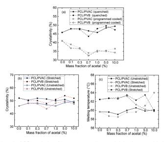
Fig. 6 DSC analysis of program cooling and injection moulded specimens. (a) Crystallinity calculated from the melting enthalpy  $(X_c^*)$ of program cooling (10 °C min<sup>-1</sup>) and injection moulded samples; (b)  $X_c^*$  and (c) melting temperature of injection sample (quenched).
