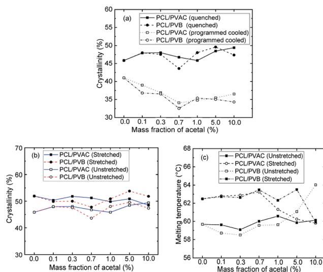
Fig. 6 DSC analysis of program cooling and injection moulded specimens. (a) Crystallinity calculated from the melting enthalpy ( $X_c^*$ ) of program cooling ( $10\text{ }^{\circ}\text{C min}^{-1}$ ) and injection moulded samples; (b)  $X_c^*$  and (c) melting temperature of injection sample (quenched).
