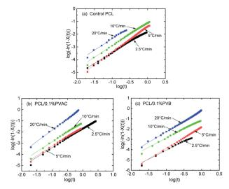
Fig. 8 Avrami plots under various cooling rates for control and nucleated PCI
