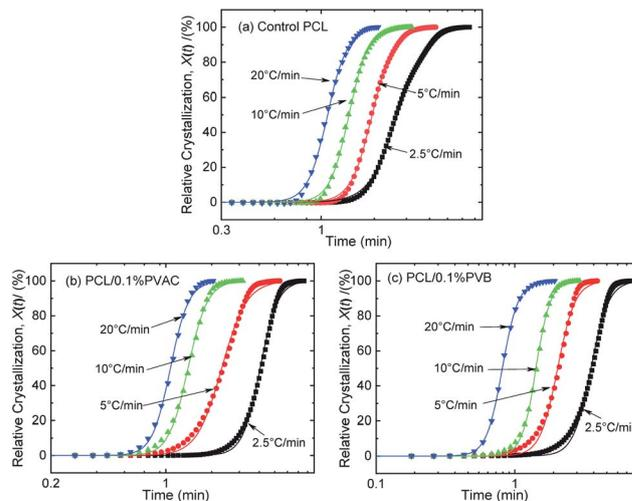
Fig. 9 Relative crystallinity versus time for (a) control PCL, (b) PCL/0.1%PVAC, and (c) PCL/0.1%PVB.
