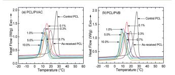
Fig. 3 DSC curves of (a) PCL/PVAC and (b) PCL/PVB blends under a cooling rate of 10 °C min<sup>-1</sup>.
