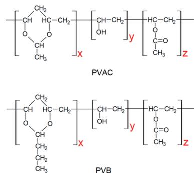
Fig. 1 Molecular structures of PVAC and PVB.
