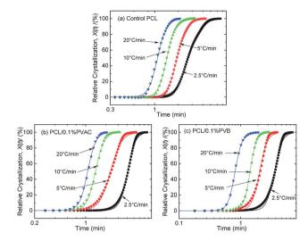
Relative crystallinity versus time for (a) control PCL, (b) PCL/ 0.1%PVAC, and (c) PCL/0.1%PVB.
