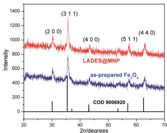
Fig. 2 X-ray diffraction pattern of LADES@MNP and  $\text{Fe}_3\text{O}_4$ . The bottom row of tick marks shows standard magnetite pattern (COD 9006920).
