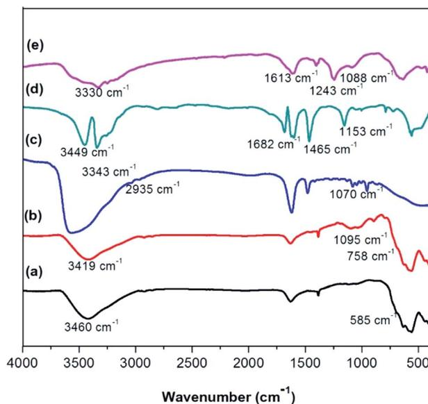
Fig. 1 FT-IR spectrum of  $\text{Fe}_3\text{O}_4$  (a),  $\text{SiO}_2@\text{Fe}_3\text{O}_4$  (b),  $(\text{CH}_2)_3\text{Cl@SiO}_2@\text{Fe}_3\text{O}_4$  (c),  $[\text{Urea}]_4[\text{ZnCl}_2]$  (d), and LADES@MNP (e).
